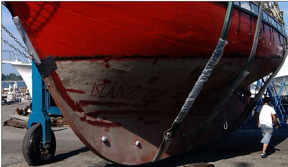
Figure 14: Keel after extension
