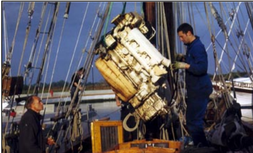
Figure 7: MTU with 147 HP; removal for overhaul in June 2004
