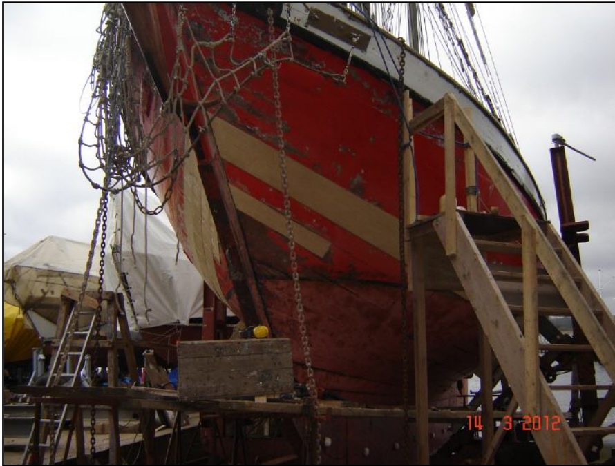
Figure 4: Renewed planking on the port side
