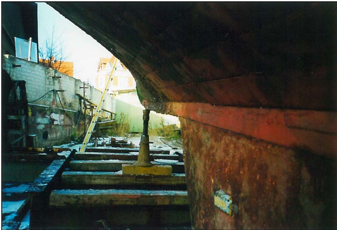
Figure 11: Keel before extension
