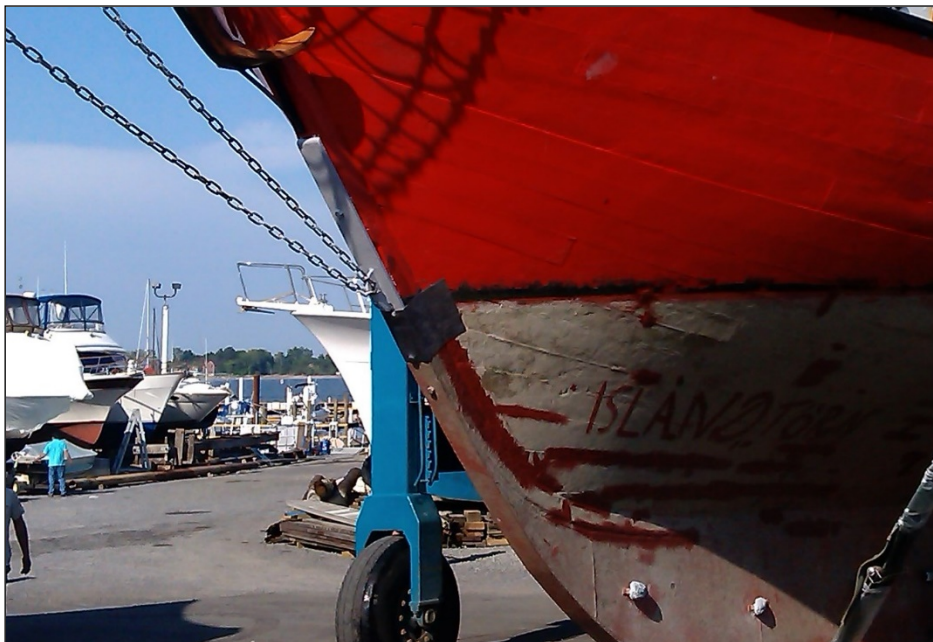
Figure 6: Stem fitting pinned with application of lead
