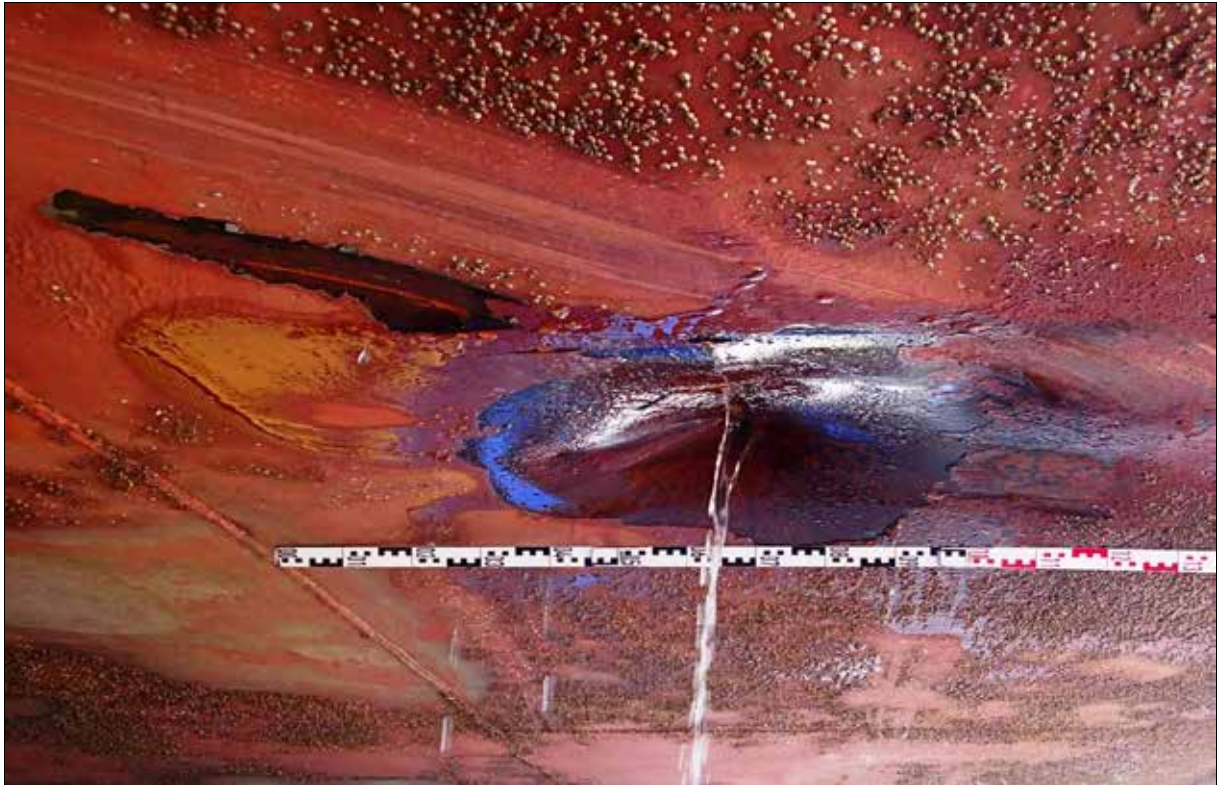
Figure 12: Leak in the bottom of the PONTON 1
