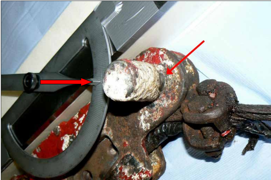
Figure 26: Determination of the angle of the attachment pressure points of the hook on the davit head of 36°
