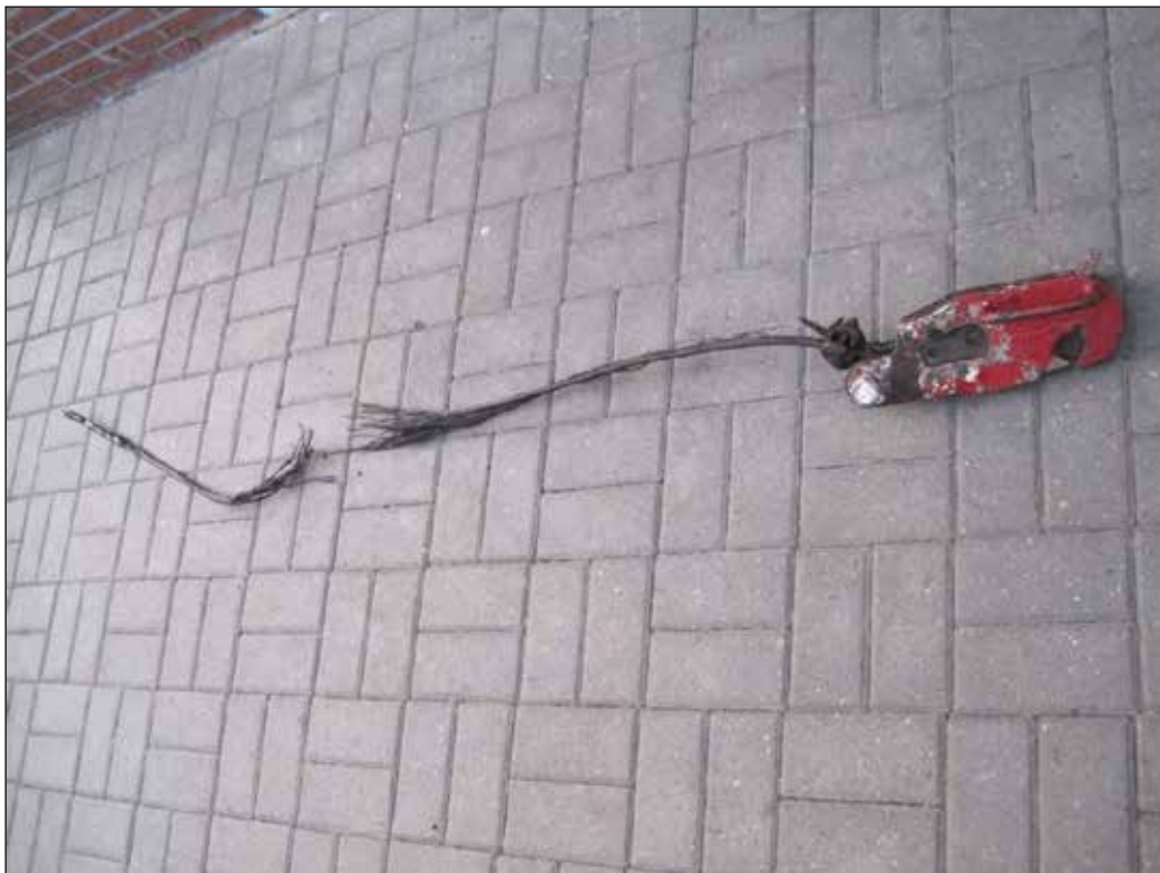
Figure 22: Hook with parted cable end
