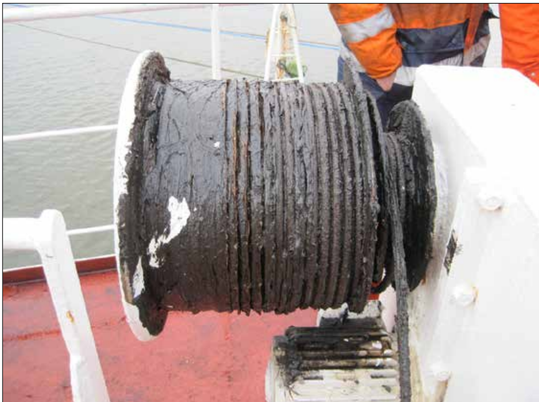
Figure 15: Winch with heavily greased cable
