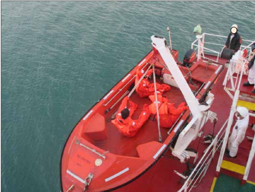
Figure 4: Start of manoeuvre; davit system still retracted
