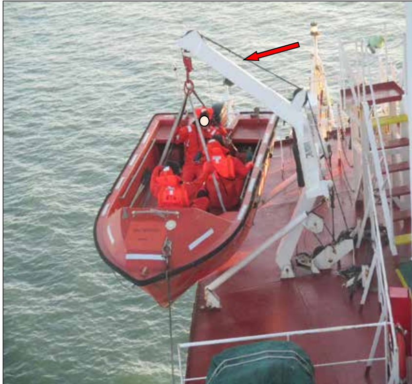
Figure 28: Approximate position of the cable failure immediately before the accident
