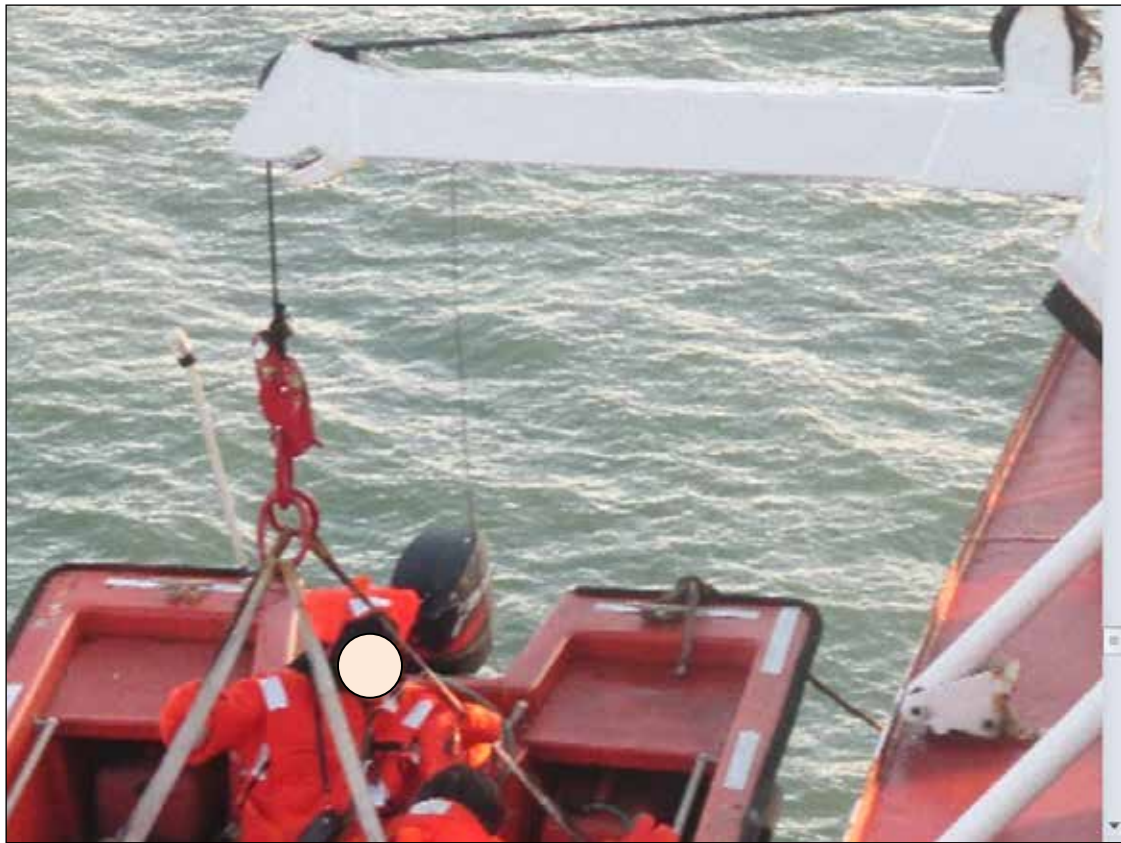
Figure 25: Photograph taken by the crew before the accident. That the cable was mounted improperly on the hook is confirmed here. Analysis of the photographs revealed that the attachment point of 36° on the davit head also seems credible
