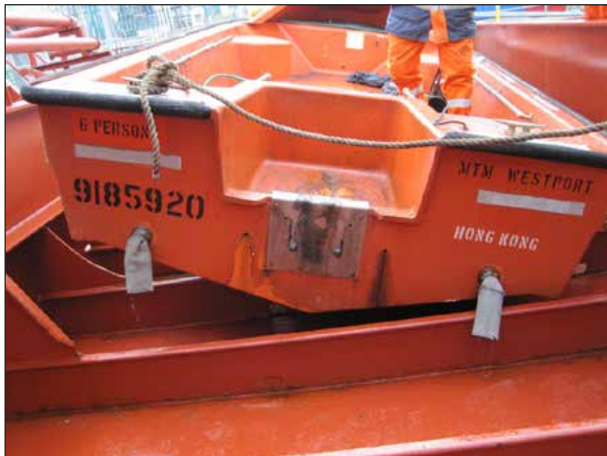
Figure 21: Rescue boat – view from aft with absent outboard engine
