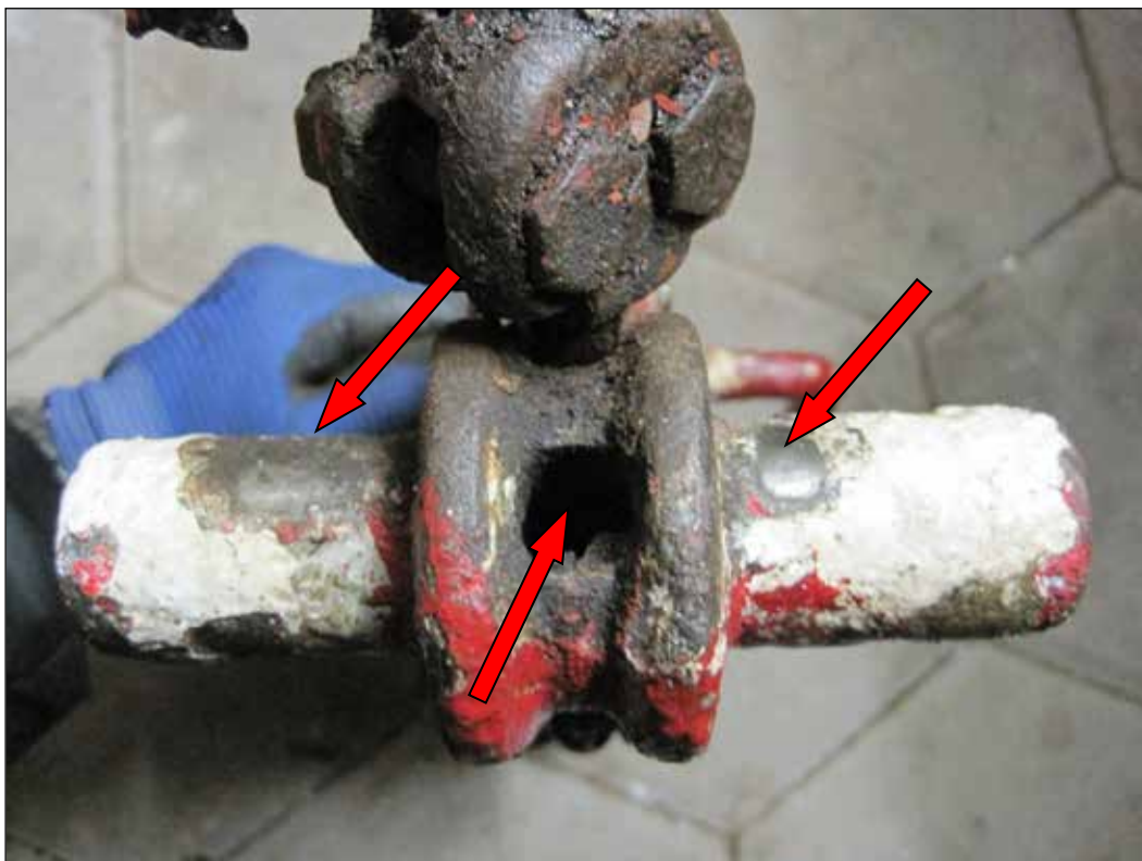
Figure 24: Cable mounted improperly on the hook. The 12-mm diameter cable should have been passed through the middle hole in the hook. Laterally, the pressure marks are visible under 36° from the vertical plane
