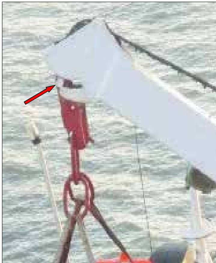
Figure 35: Immediately before the accident – the hook cannot retract further because the cable clamp is resting against the upper guide pulley
