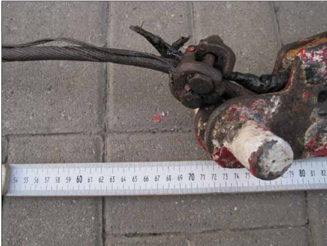
Figure 23: Inclined cable clamp
