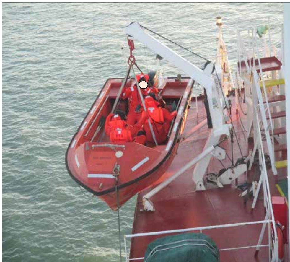
Figure 7: Davit system retracted with the boat
