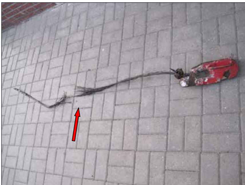
Figure 29: Position of the cable failure 700 mm above the hook
