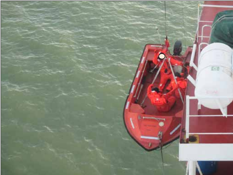
Figure 6: Boat is hoisted out of the water until the davit head is reached
