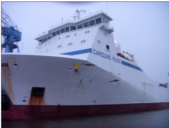
Figure 4: Bow damage on the CAROLINE RUSS
