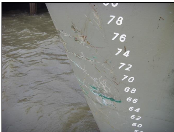
Figure 6: Bow damage (BARENT ZANEN)
