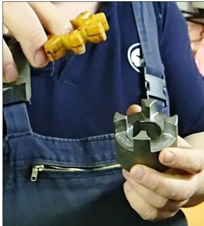
Figure 13: Section of coupling with plastic buffer removed
