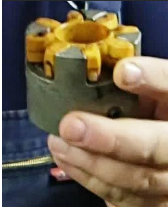
Figure 12: Section of coupling with plastic buffer
