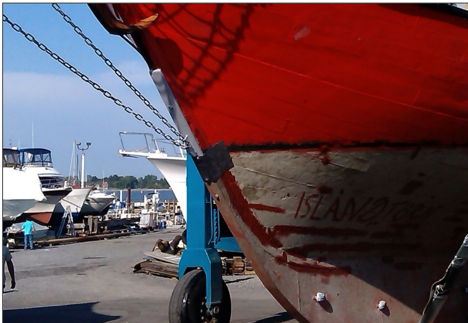
Figure 6: Stem fitting pinned with application of lead
