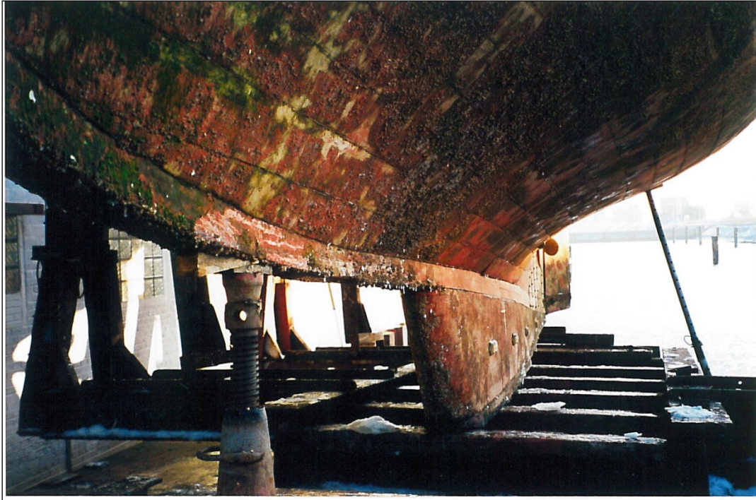
Figure 10: Keel before extension
