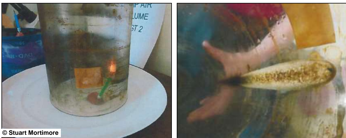
Figure 89: Test to establish the internal flammability of the ceiling lighting 61
