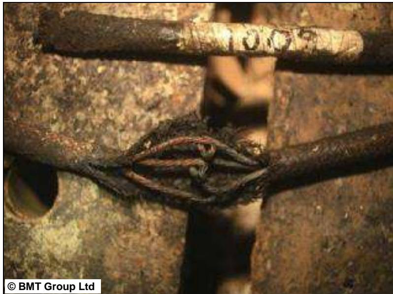
Figure 70: Example of metal conductor within the insulation 43
