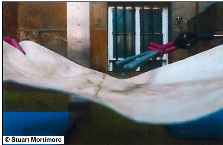
Figure 94: Test setup to establish the flammability of a tarpaulin 67
