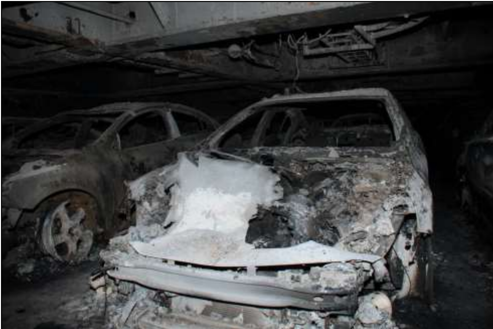
Figure 109: Car 4 C below the cable rack with fire pattern from the engine compartment
