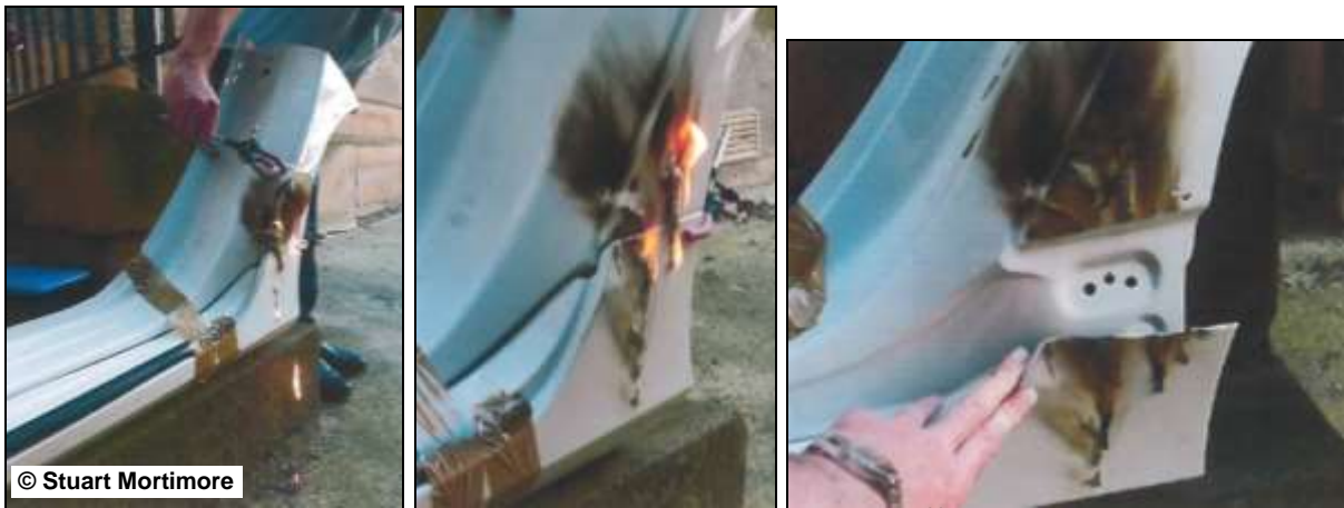
Figure 90: Ignition of the door sill (1) 62
