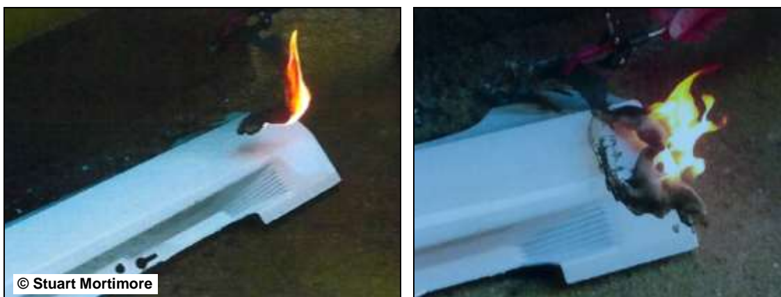
Figure 91: Ignition of the door sill (2) 63
