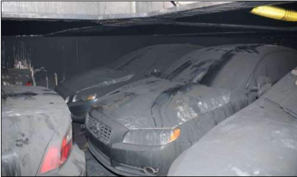
Figure 9: Cars severely fouled by soot
