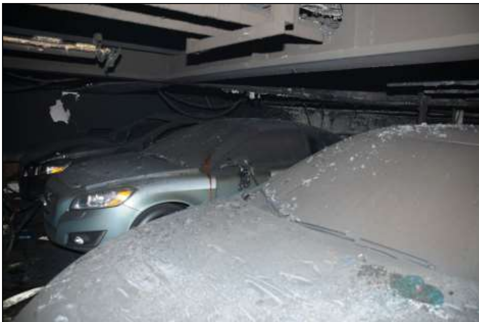
Figure 50: Various traces of damage to adjacent vehicles
