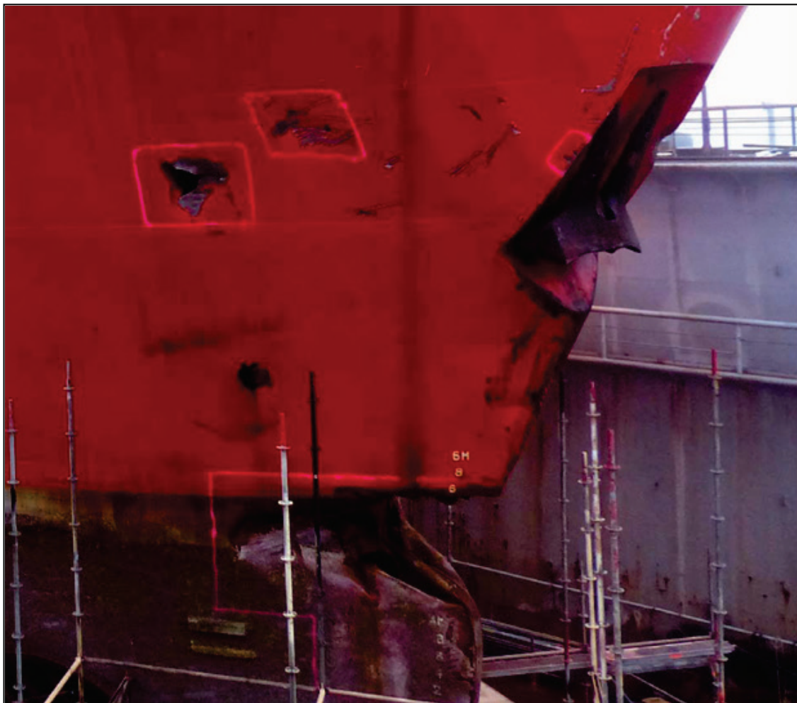
Figure 19: Damage to the bow
