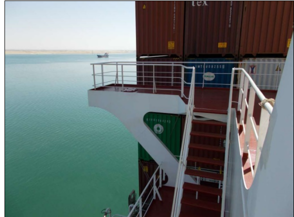
Figure 16: Transverse passageway on the starboard side
