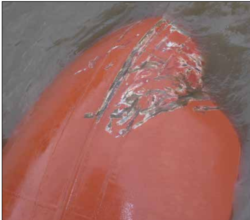
Figure 8: Damage to the CORAL IVORY's bulbous bow
