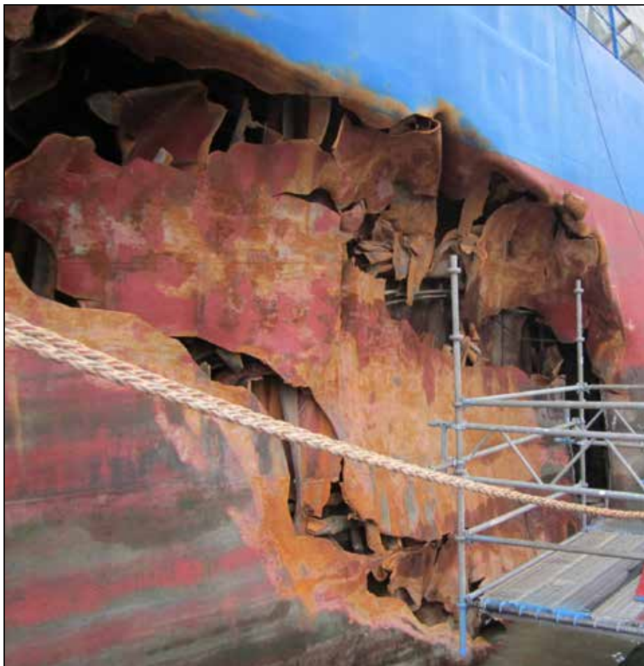
Figure 41: Hole in the SIDERFLY's shell plating (port side)
