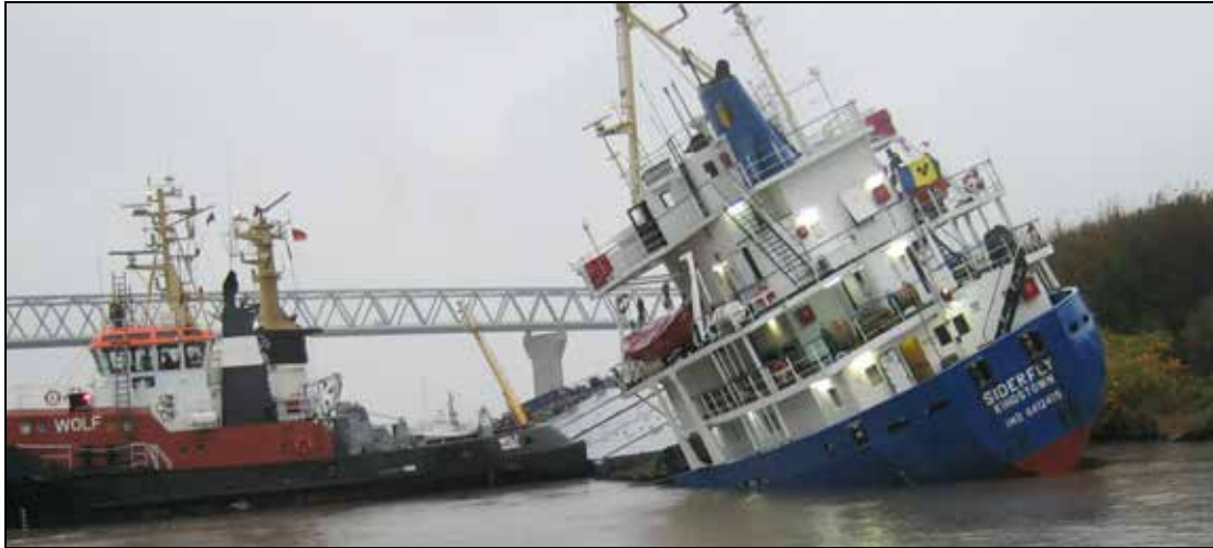
Figure 48: Tug-induced load on the hatch cover
