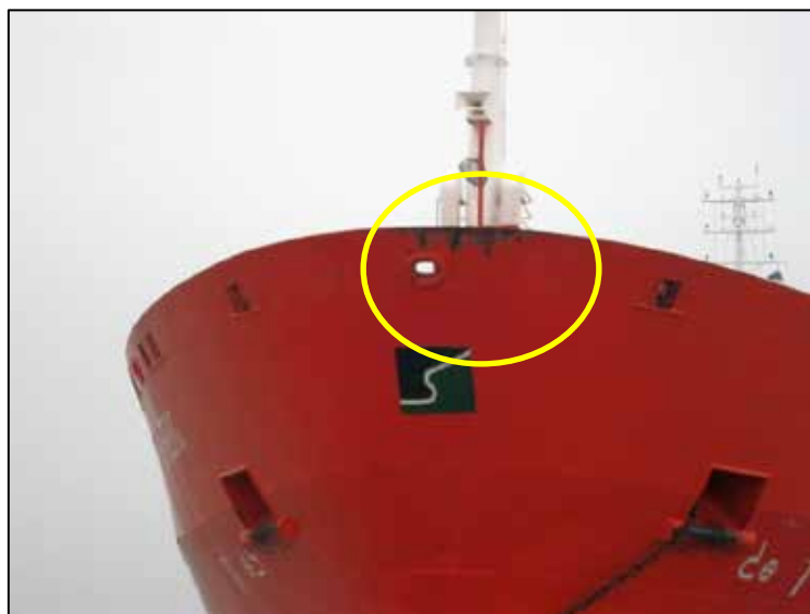
Figure 5: STENBERG with minor damage to her bow
