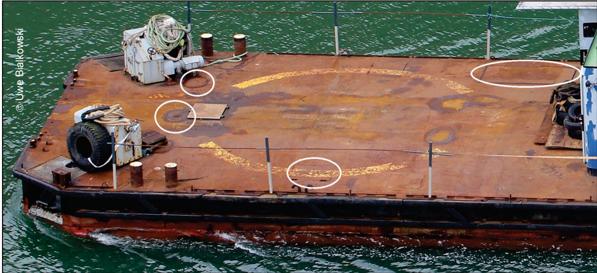
Figure 13: Deck openings on the fore section
