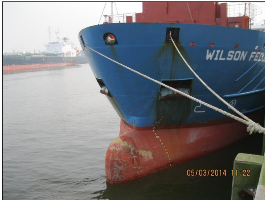
Figure 21: Paint abrasions on the WILSON FEDJE's bulbous bow
