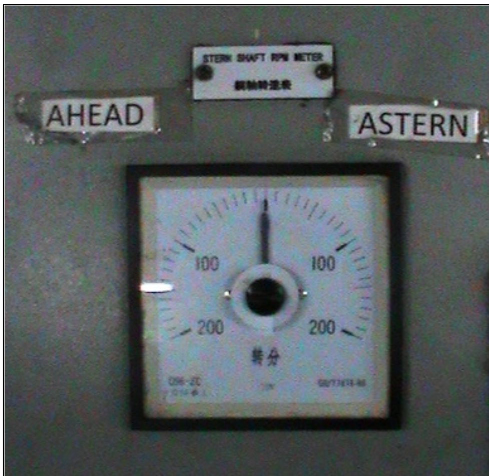
Figure 13: Indicator for rated speed and direction of rotation of the propeller in the ECR
