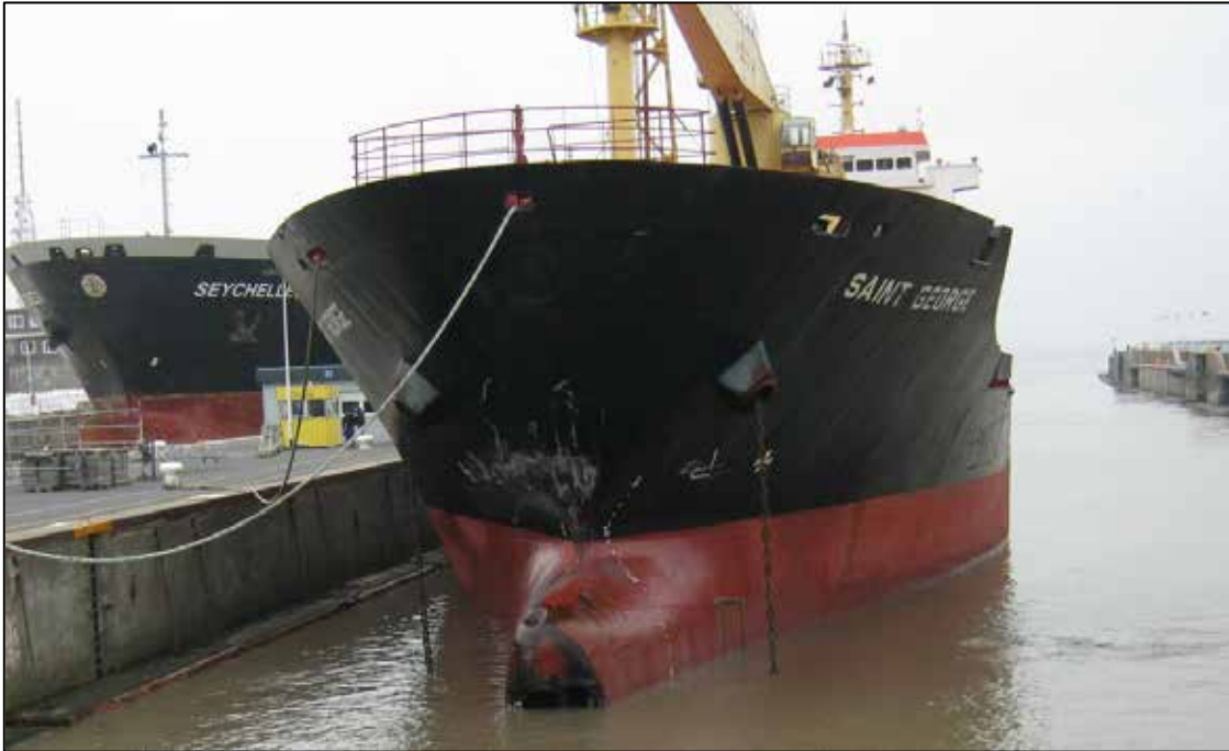
Figure 3: Damage to the fore section
