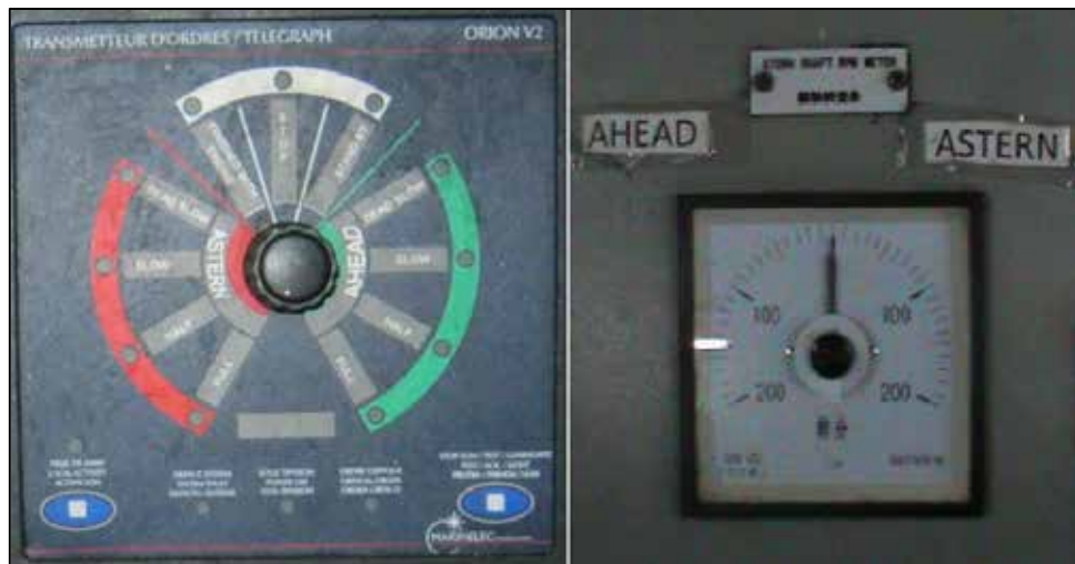
Figure 21: Comparison between the engine order telegraph and indicator showing the direction of rotation
