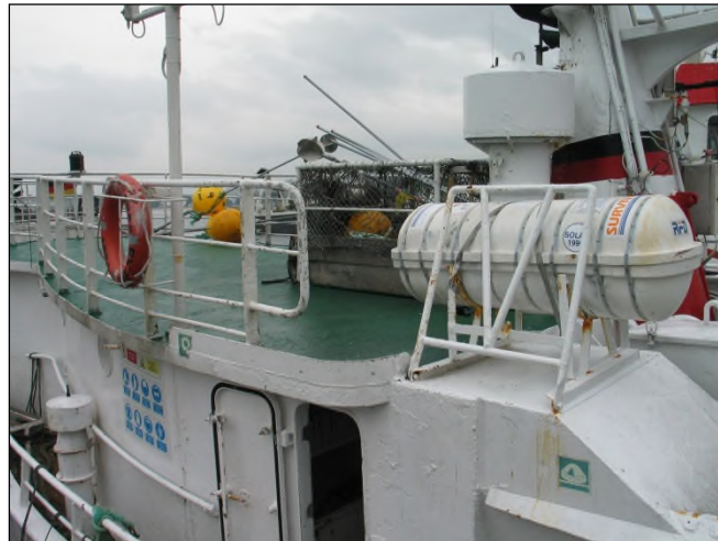
Figure 3: Missing guard rail on the observation deck
