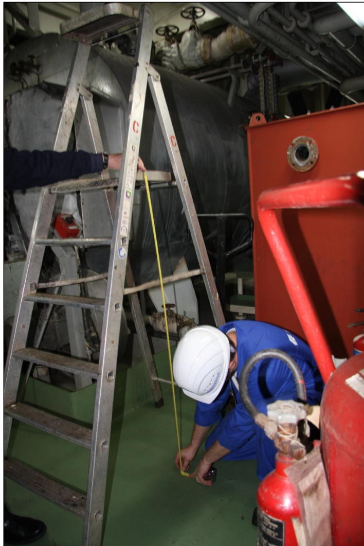
Figure 13: Position of the ladder at the time of the accident (reconstruction)
