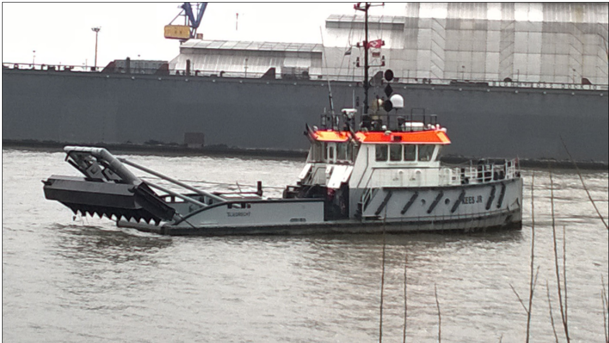
Figure 3: Bed leveller KEES JR
