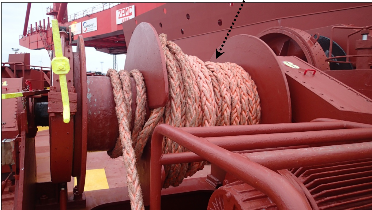
Figure 8: Winch holding the parted line
