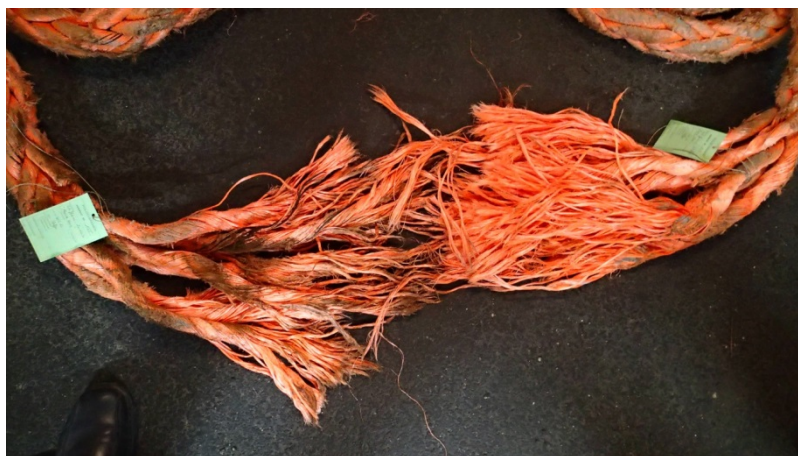
Figure 6: Line's point of failure
