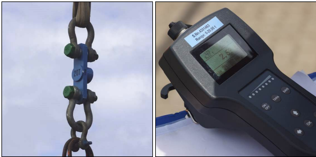
Figure 12: Special scale and device for wirelessly recording measurements
