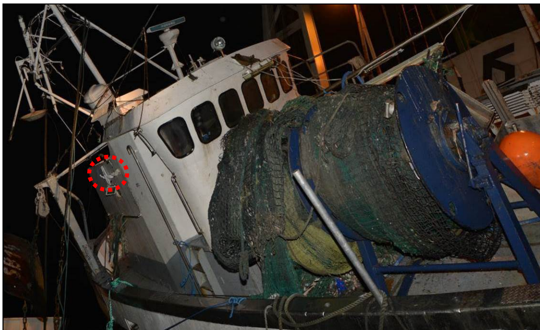
Figure 27: FV CONDOR immediately after salvage (empty EPIRB mount visible)
