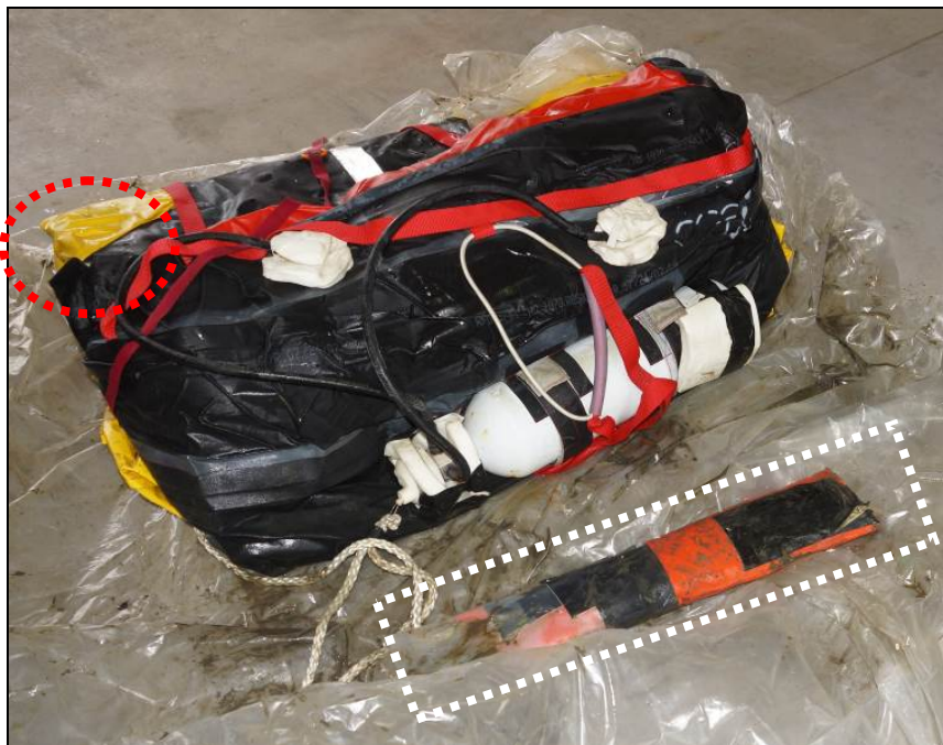
Figure 49: Intended position of the opening in the container compared to position of the painter satchel after removal of the liferaft's protective plastic covering
