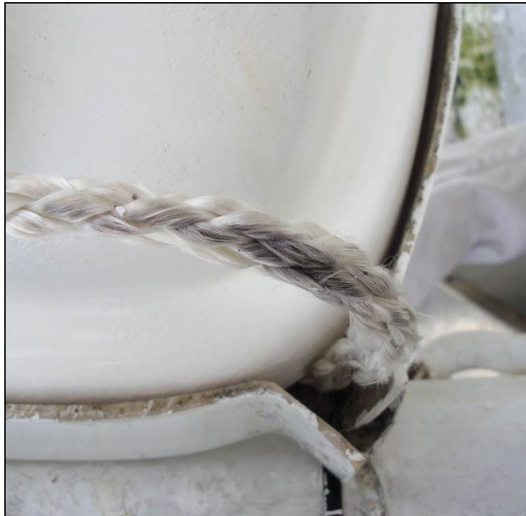
Figure 41: Close-up of the liferaft's container (opening for the painter/release cord)
