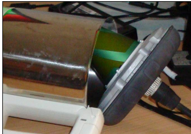
Figure 66: Shielding the antenna with a metal container
