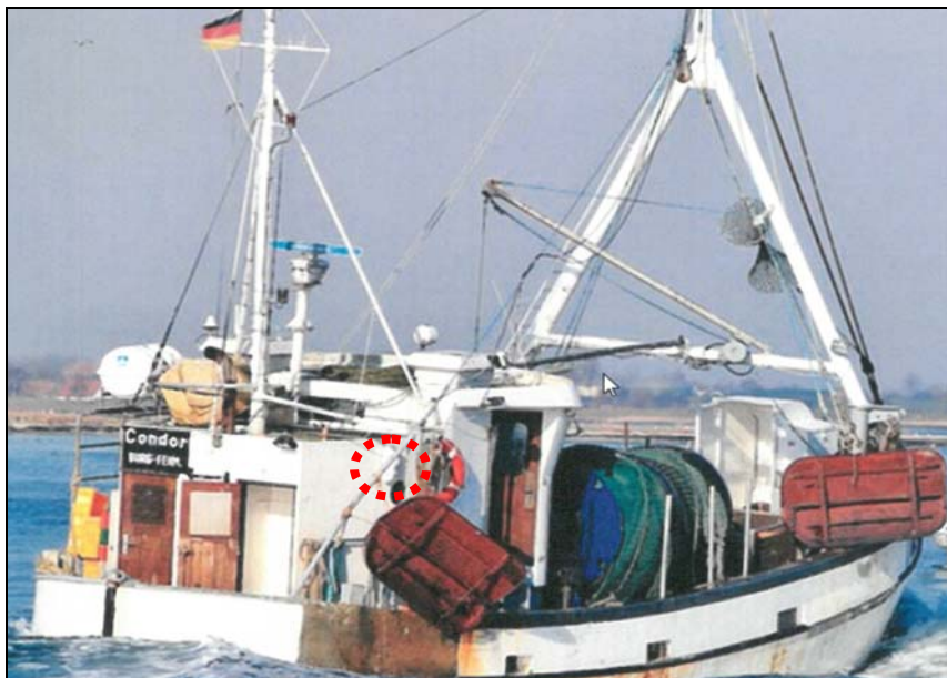
Figure 25: FV CONDOR – mounting position of the EPIRB
