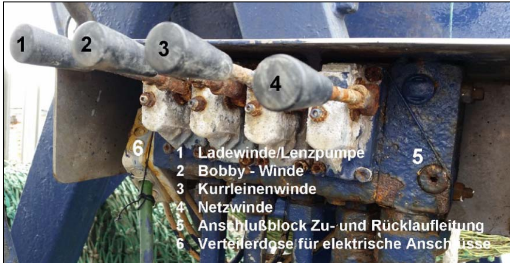
Figure 99: Winch control position on deck
