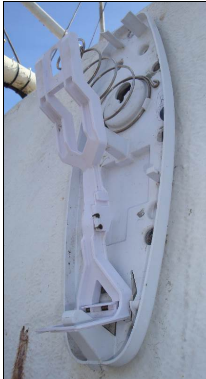
Figure 28: Open EPIRB mount (starboard side of fishing vessel – wheelhouse)
