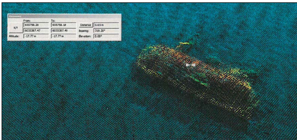
Figure 3: Sonar image of the wreck of the FV CONDOR 9
