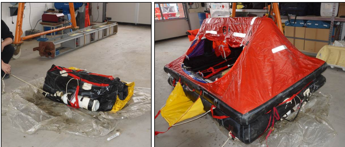
Figure 52: Manual activation of the inflation process
