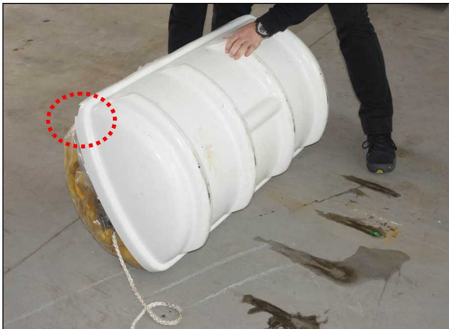
Figure 47: Liferaft tipped carefully out of the container
