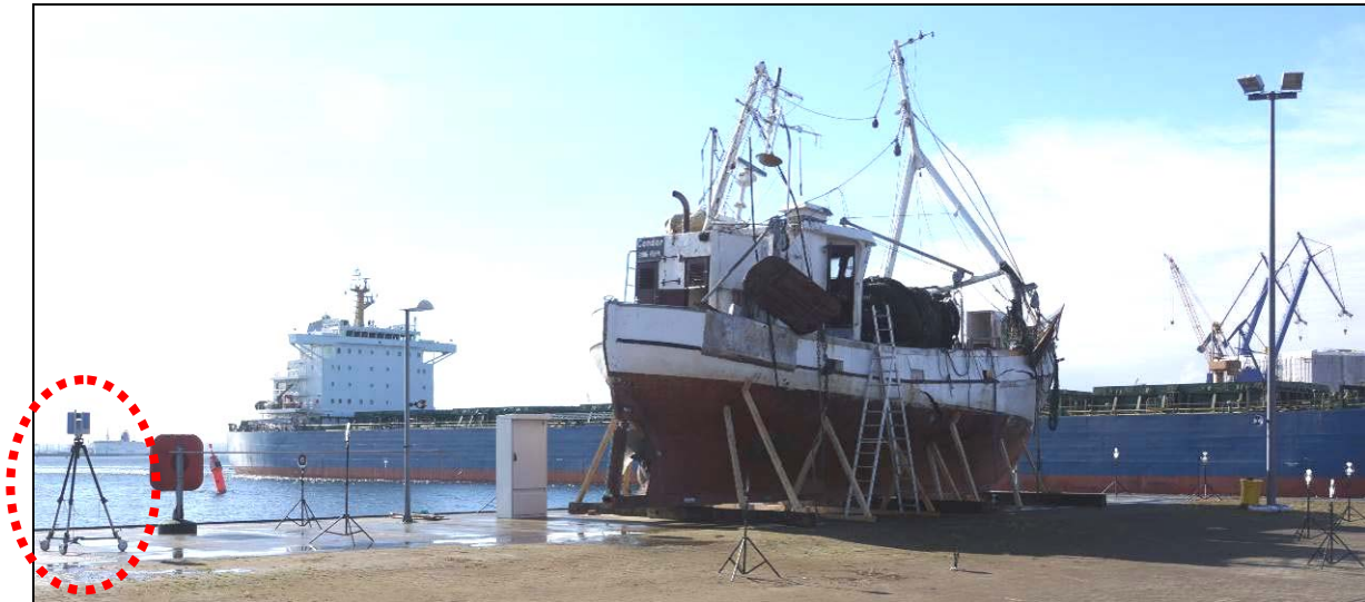
Figure 10: 3D laser scan of the FV CONDOR by LKA Hamburg on 15 March 2016
