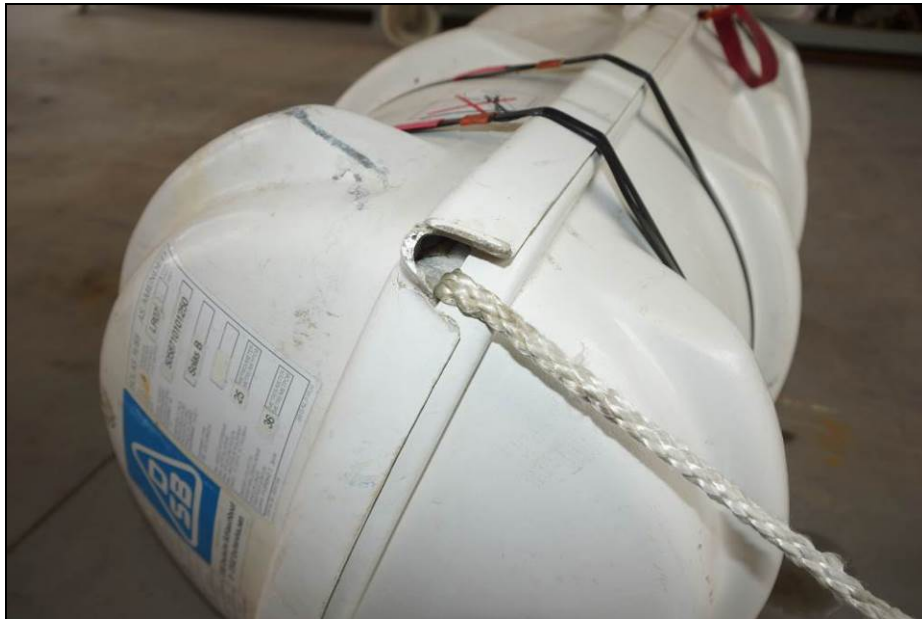
Figure 45: Painter/release cord's exit point from the container (cord cannot be pulled out with muscular force)
