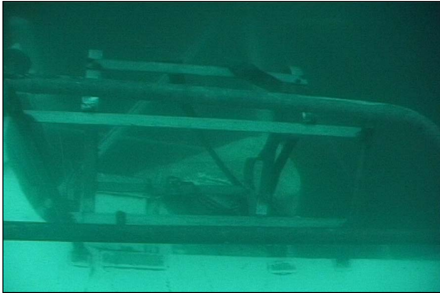
Figure 37: Empty liferaft mount (extract from the DENEb's dive video – 12 February 2016)
