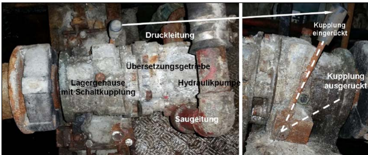
Figure 97: Winch hydraulic pump with drive
