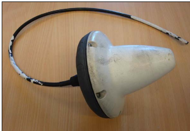
Figure 62: The BLE antenna exhibiting no visible damage
