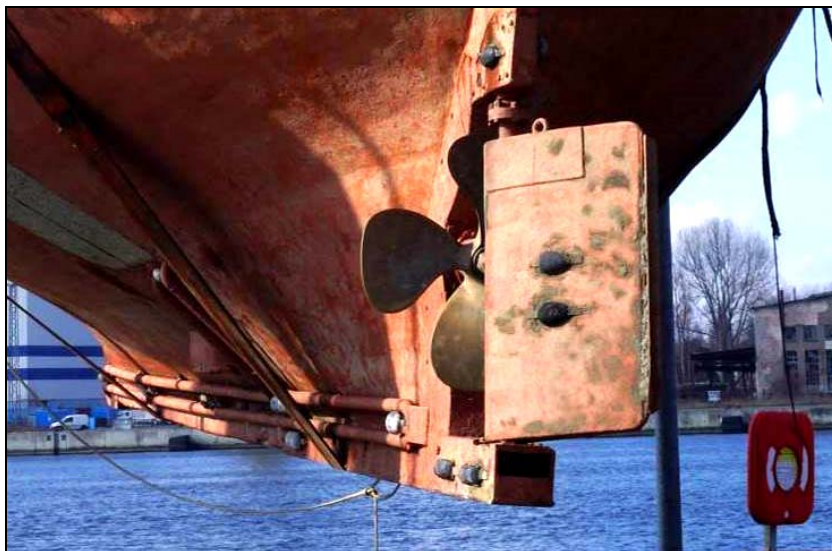
Figure 22: Position of the rudder blade (unchanged during the salvage operation)
