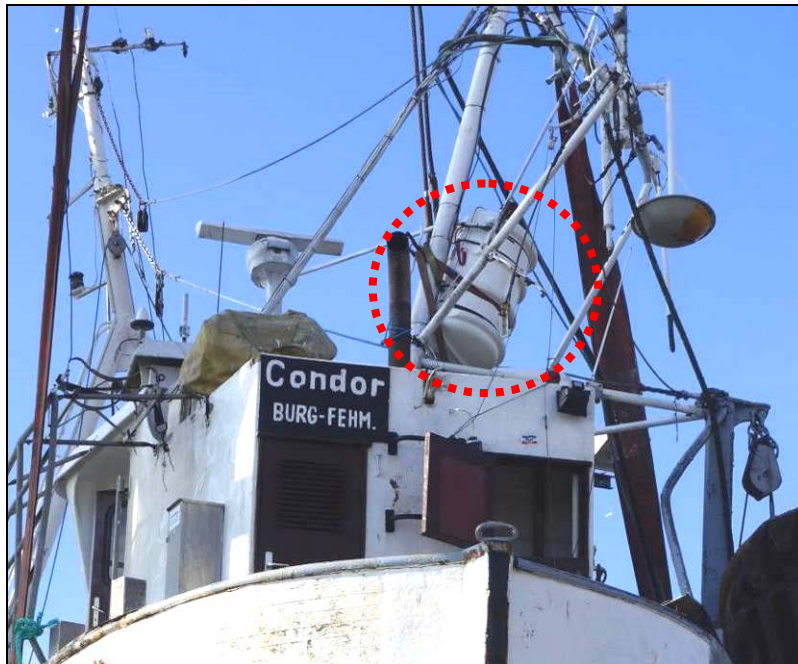
Figure 39: FV CONDOR (arrival in Rostock; liferaft provisionally attached to the mast)
