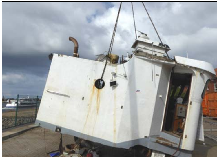
Figure 118: Weighing the entire superstructure, including toilet compartment and exhaust
