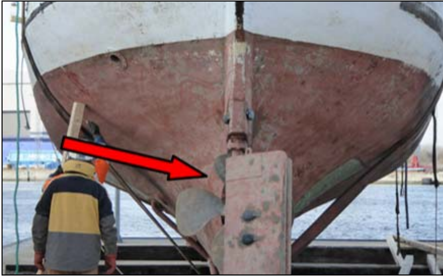
Figure 108: Position of the rudder blade at the time of the accident
