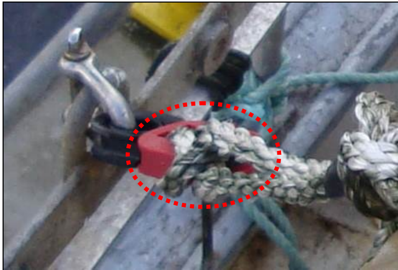
Figure 36: Close-up of painter/release cord connection with liferaft mount
