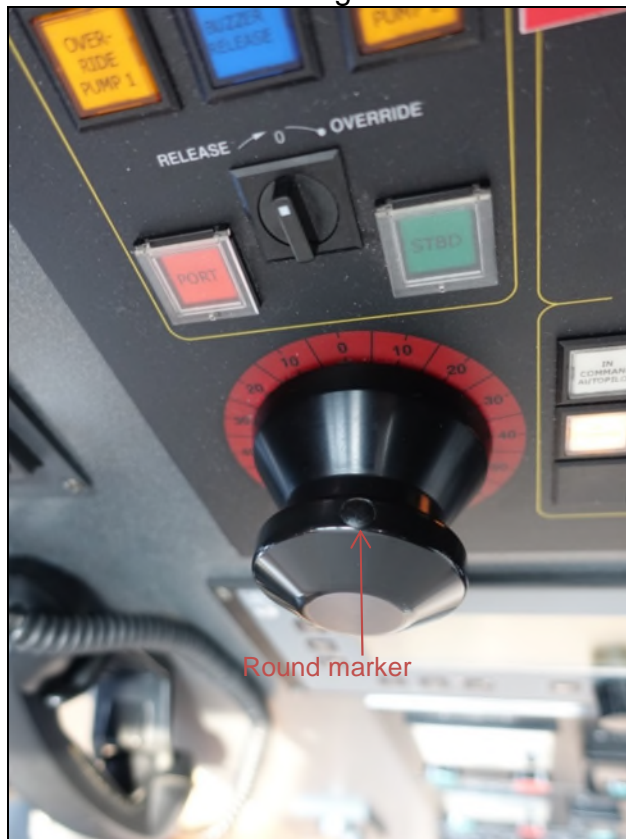
Figure 30: Manual helm with stepping amidships (0)
