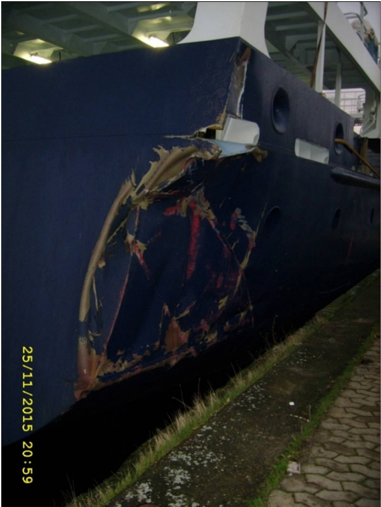
Figure 5: Damage to the EENDRACHT's aft section, Ship Safety Division (BG Verkehr)
