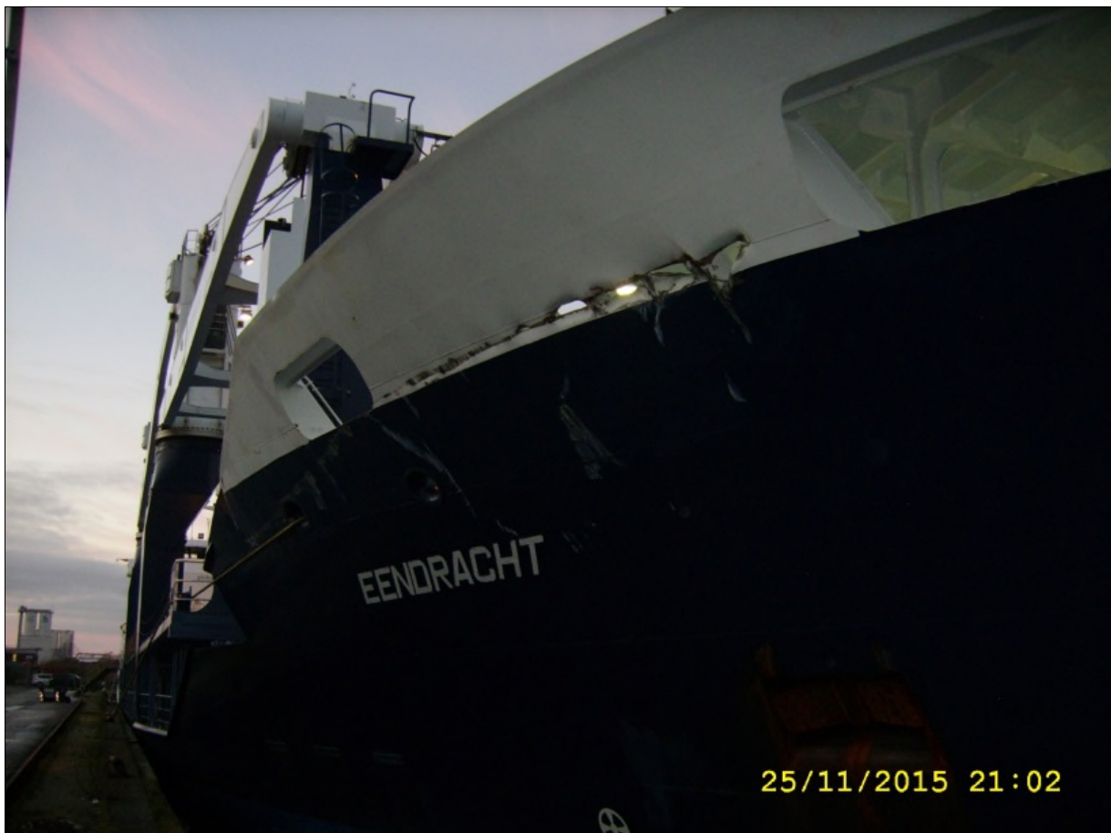
Figure 4: Damage to the EENDRACHT's fore section, Ship Safety Division (BG Verkehr)
