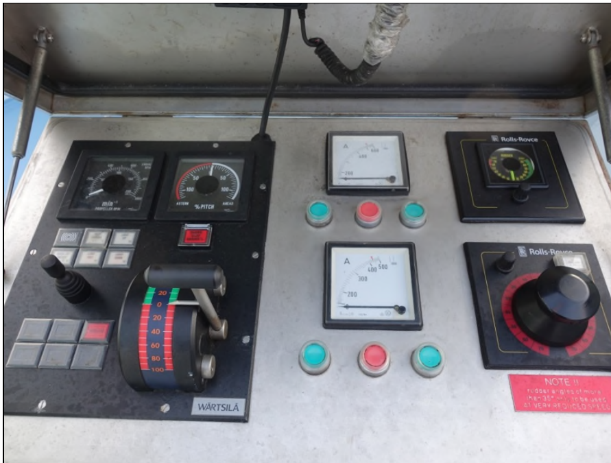
Figure 31: Wing manoeuvring platform
