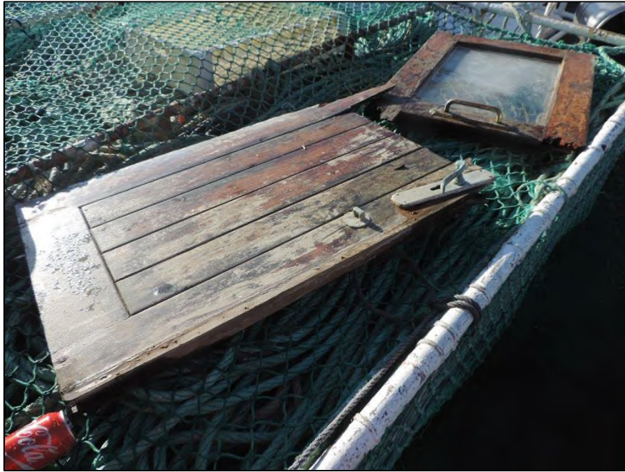
Figure 6: Destroyed wheelhouse door
