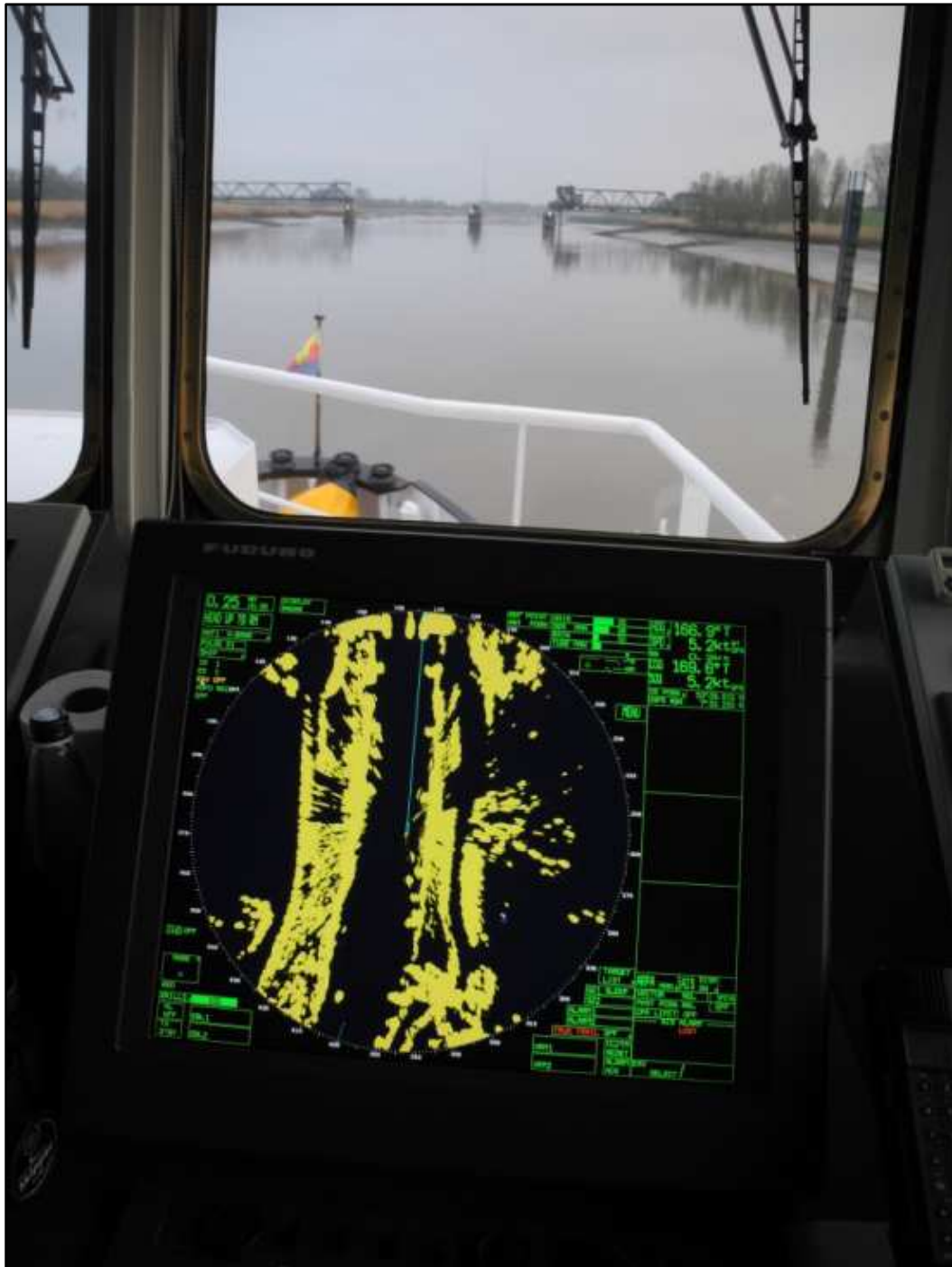
Figure 22: Friesenbrücke Bridge, range of 0.25 nm – both passages visible
