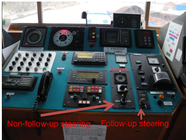
Figure 7: Follow-up and non-follow-up steering with tiller
