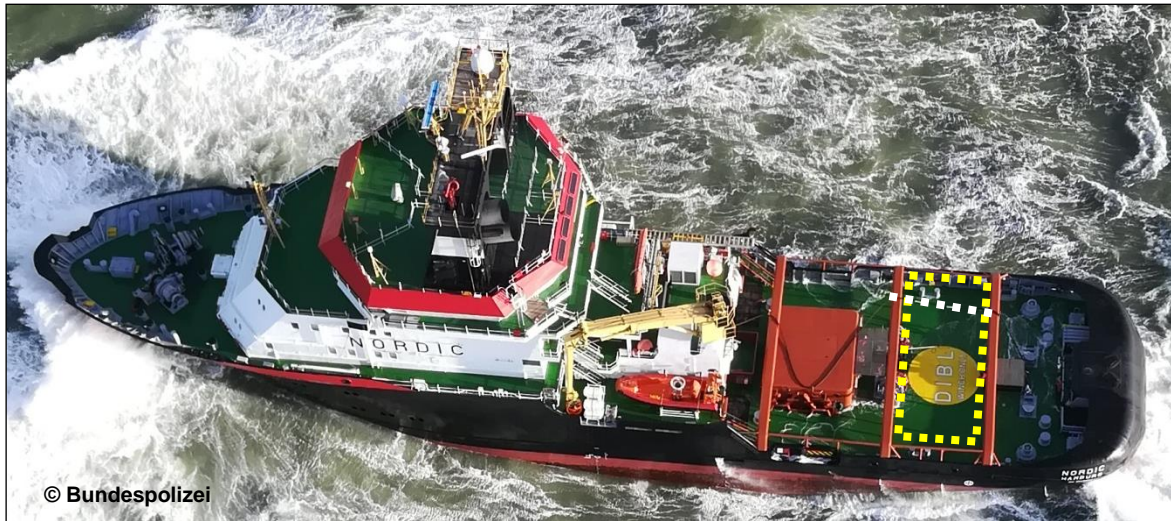
Figure 3: Emergency tug NORDIC at the day of the accident (winch area marked yellow)
