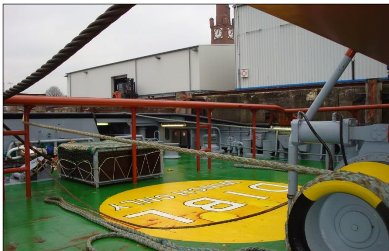
Figure 5: Restriction of the winch area by steel cross braces (partial view)
