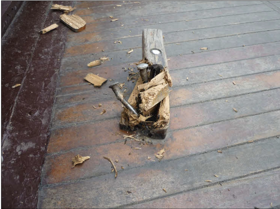
Figure 7: Destroyed wooden cleat (front view)
