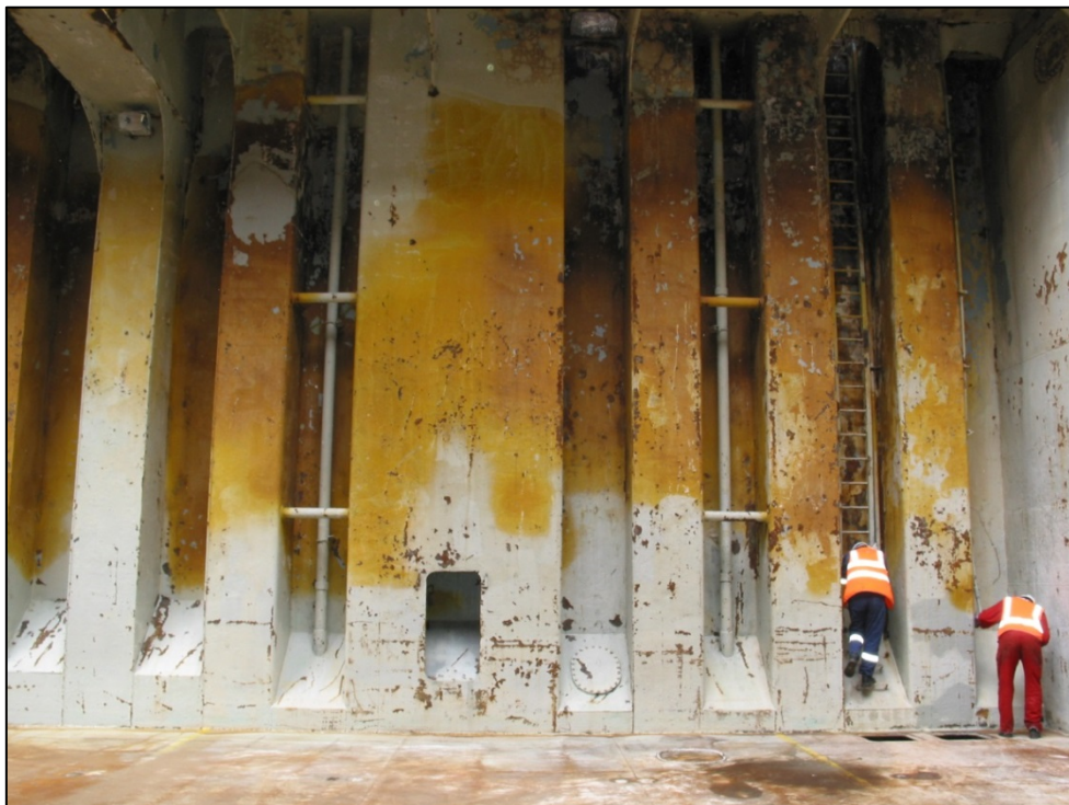
Figure 61: Cargo hold 2's lower hold, port side of aft edge with discolouration
