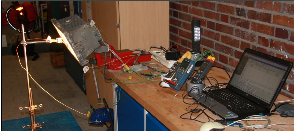
Figure 48: Measurement setup for determining the surface temperature of the cargo hold light
