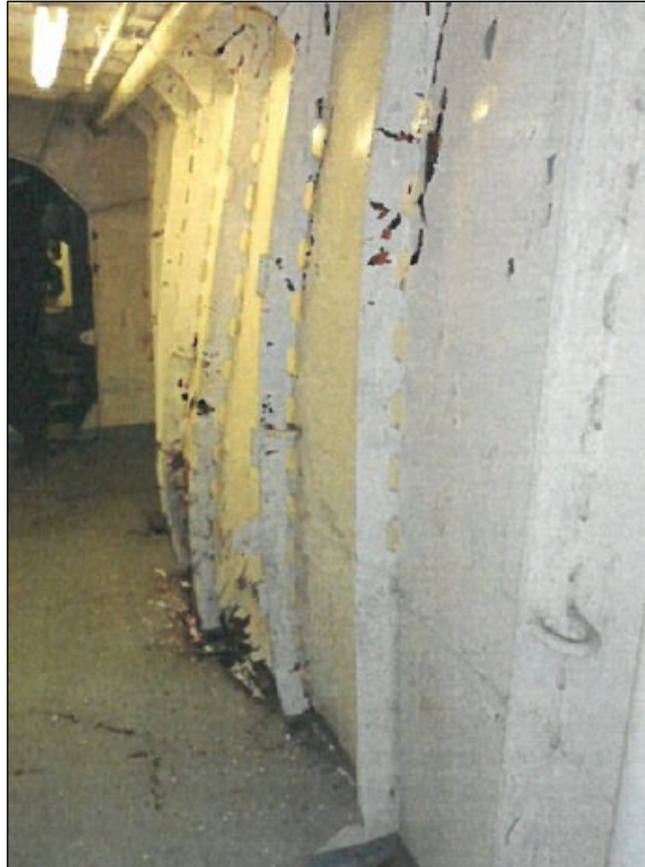
Figure 20: Damage to the MERIDIAN's starboard side...
