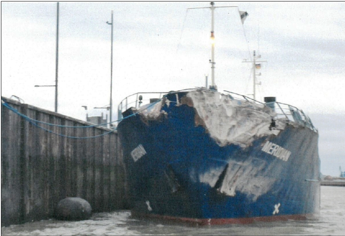
Figure 18: Damage to the MERIDIAN's bow
