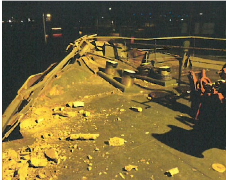
Figure 22: Damage to the MERIDIAN's fore section
