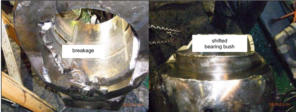
Figure 13: Connecting rod eye with breakage and laterally shifted bearing bush
