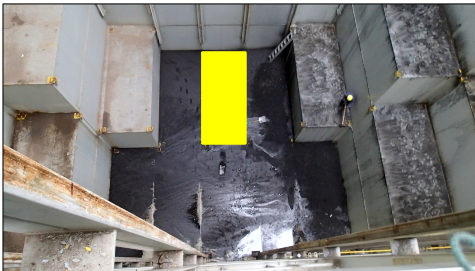
Figure 25: Example for a poorly achievable storing position of a 20-ft container
