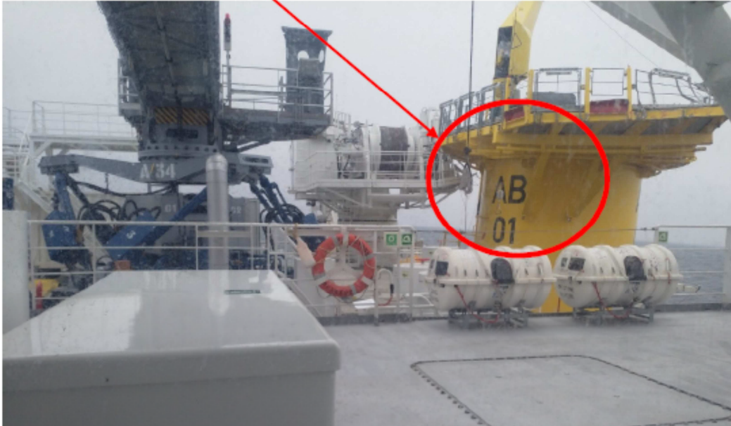
Figure 10: Allision between the shipboard crane and flange deck
