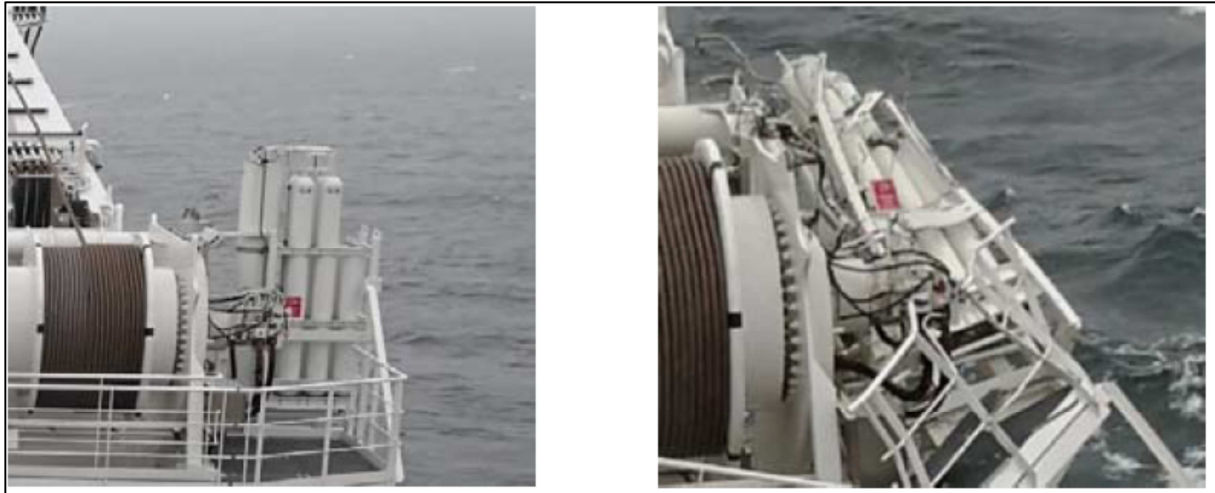
Figure 12: Shipboard crane before and after the collision
