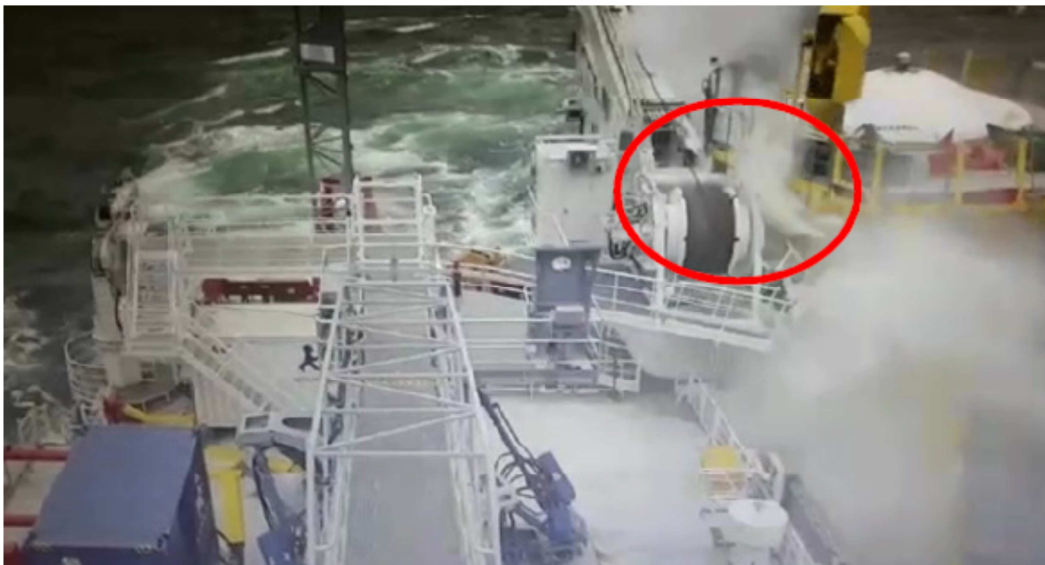
Figure 11: Damage to the nitrogen cylinder
