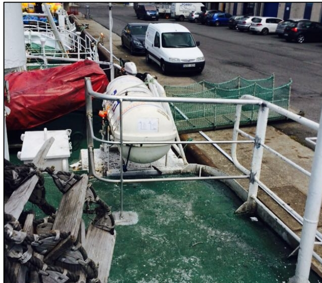
Figure 22: Additional guard rail next to the liferaft
