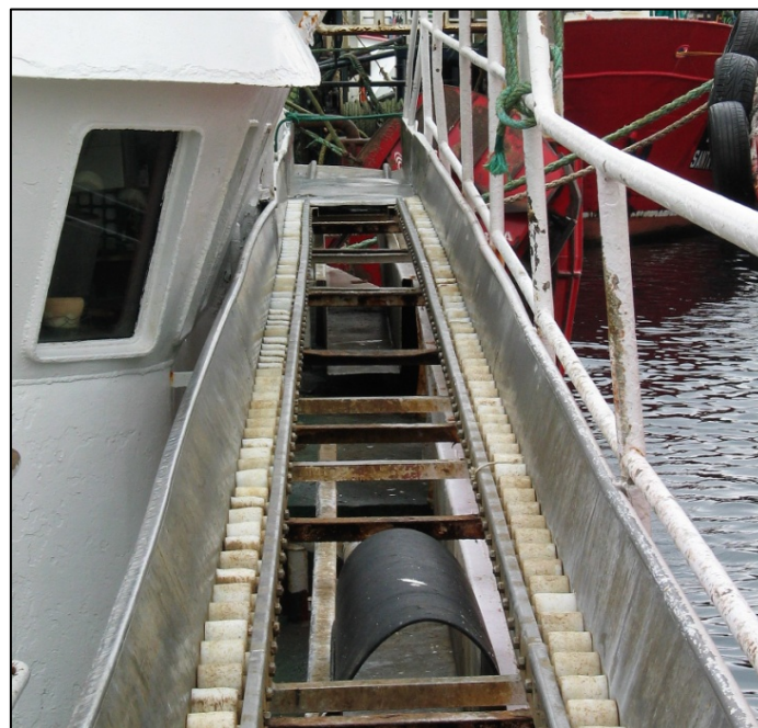
Figure 14: Shooting ramp, detailed view looking aft with rollers and cross members
