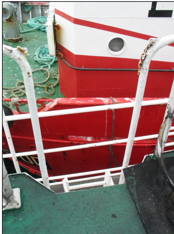
Figure 16: Opening between ladder and observation deck without securing chain
