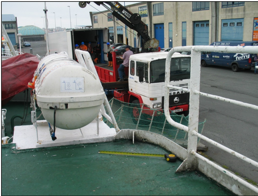
Figure 21: Unsecured area next to the liferaft
