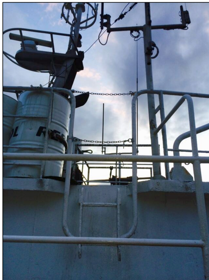
Figure 25: Ladder to observation deck with safety chains
