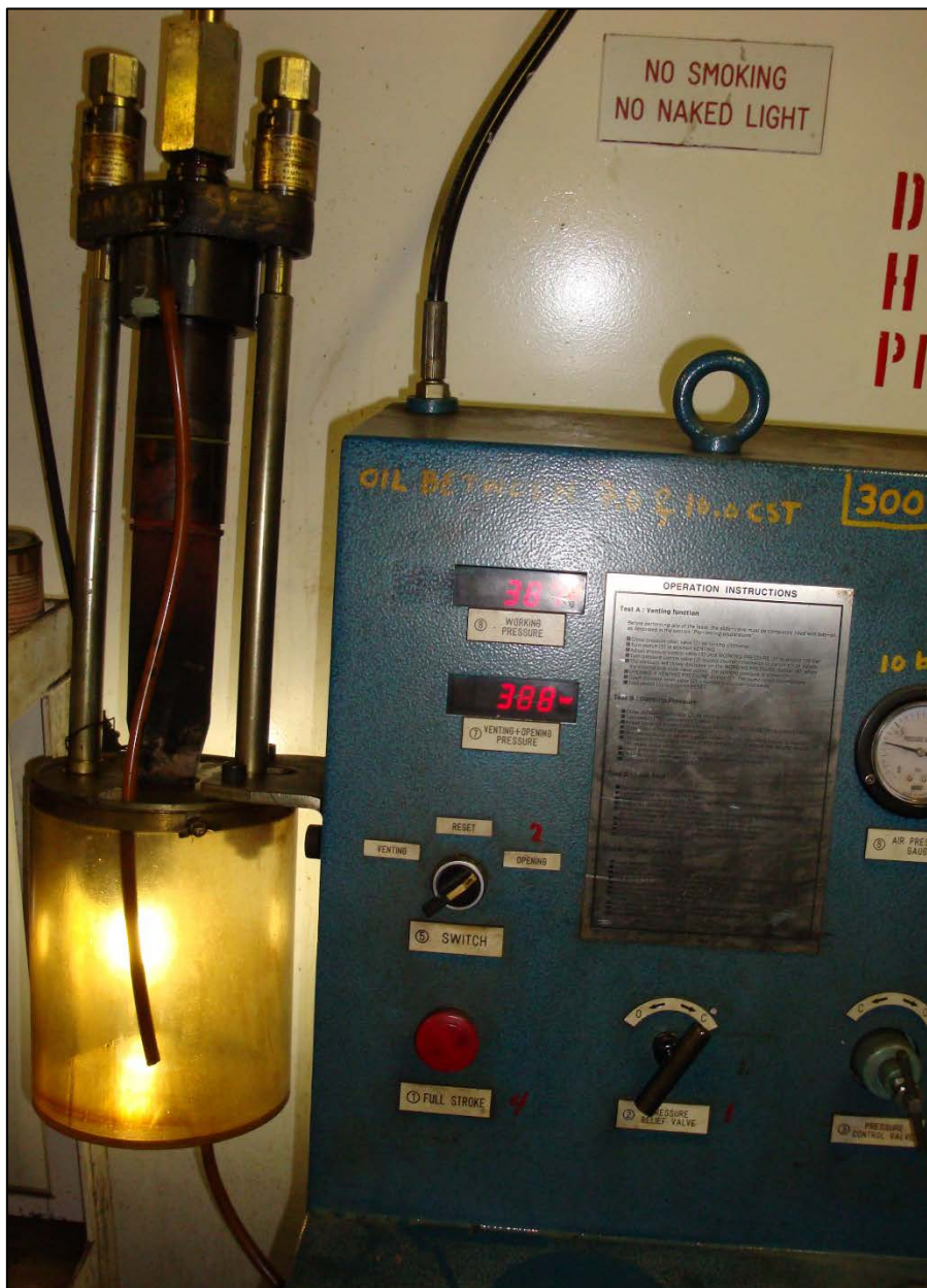
Figure 9: Rig for pressure testing injectors in the CAPE LEONIDAS's ECR
