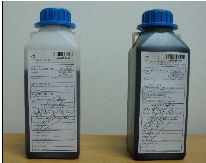
Figure 10: Fuel samples from the CAPE LEONIDAS's day tanks
