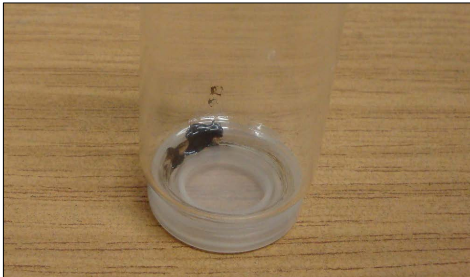
Figure 11: Secured residues from the fuel inlet of the defective injector
