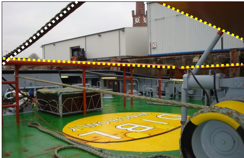
Figure 35: Winch area bounded by steel towing rails and towing cable (partial view)
