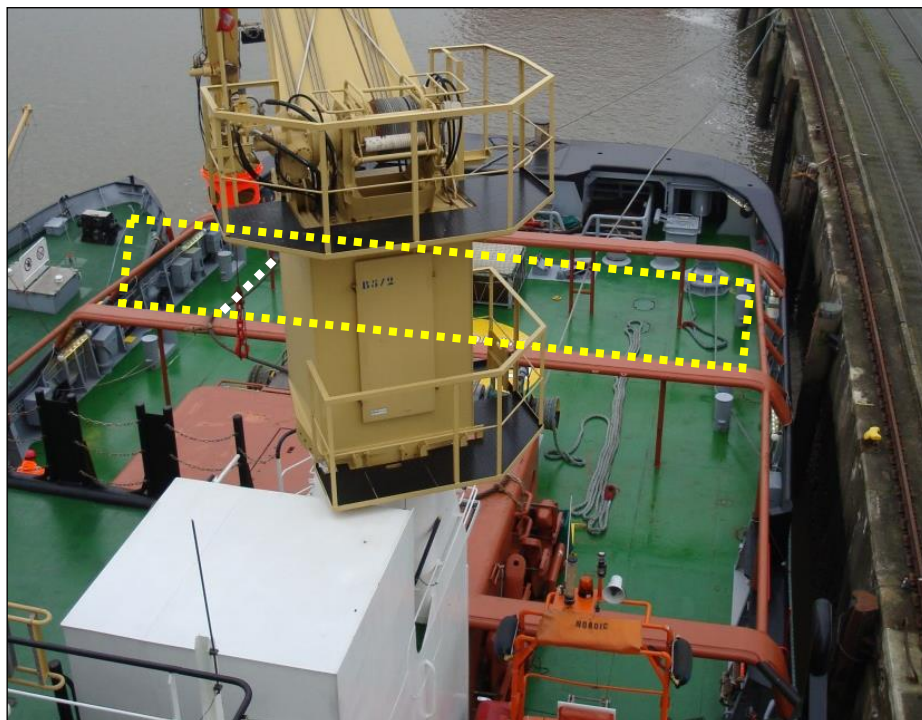
Figure 34: Lateral view of the winch area (bounded by steel towing rails and towing cable)
