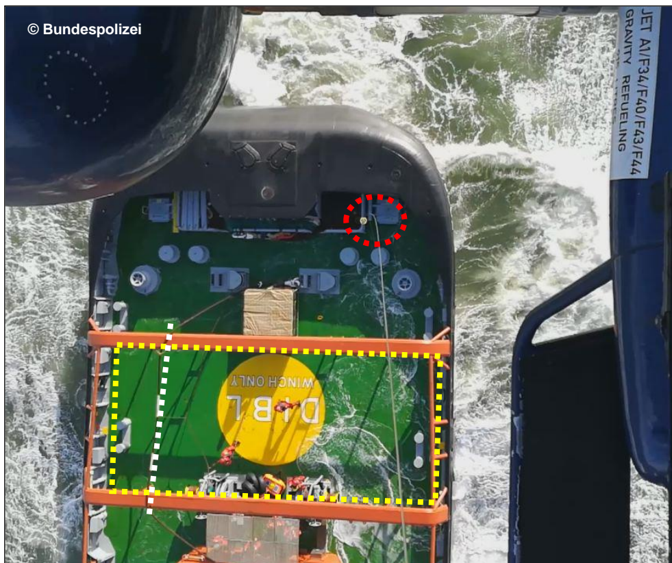
Figure 32: Attempt to lower the winch hook at the day of the accident
