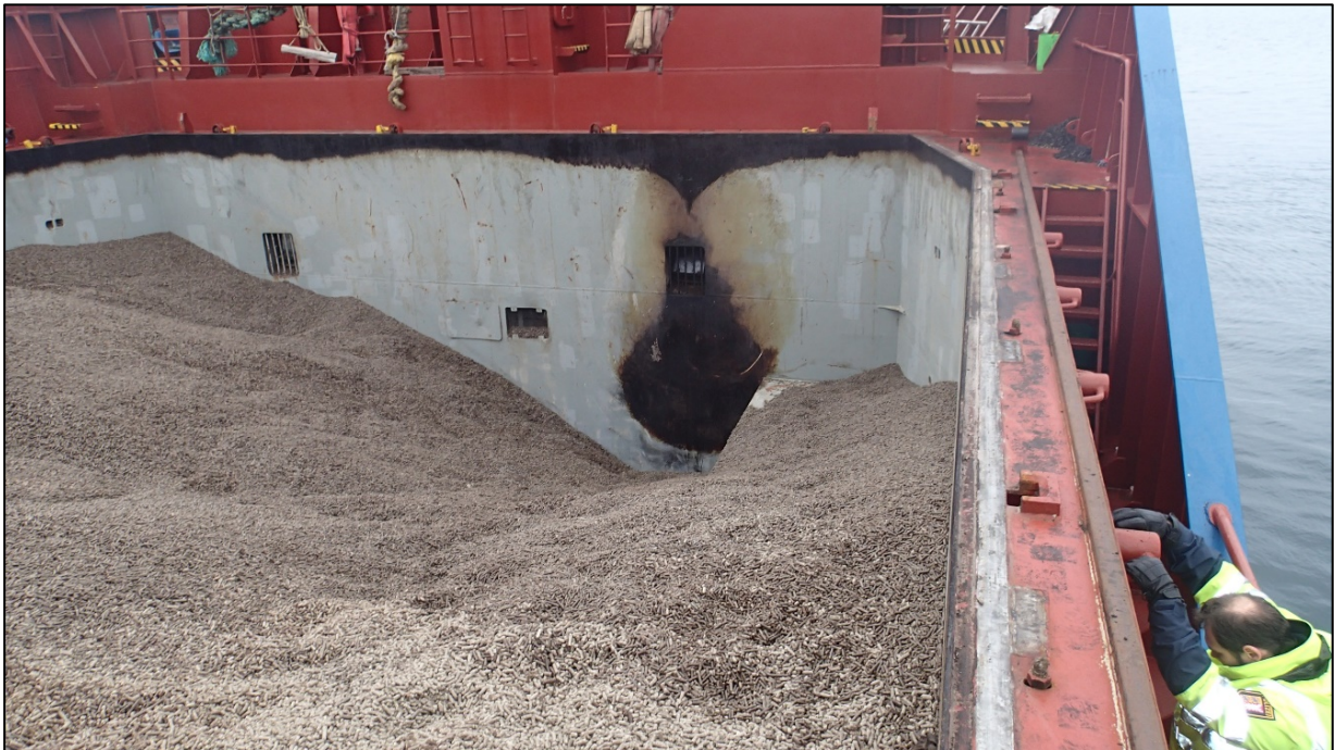
Figure 7: Area fouled by soot above the cargo and hotspot on the wing tank
