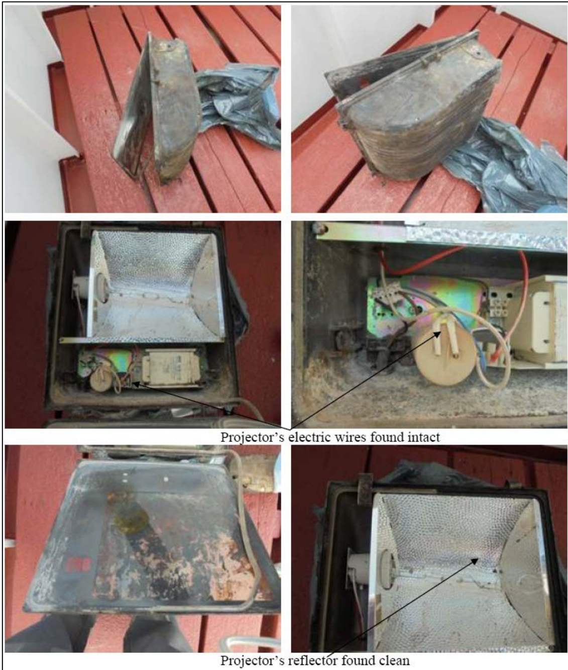
Figure 13: Starboard cargo hold lights
