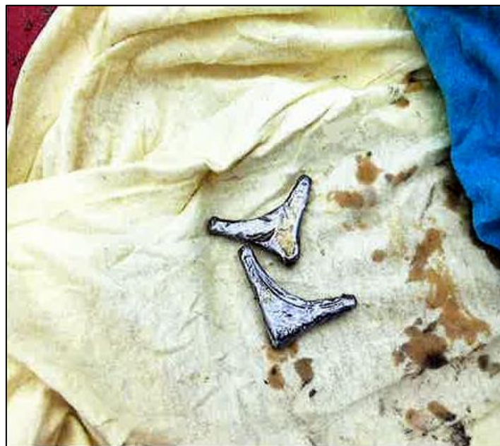
Figure 42: Fragments of the support plate found 26
