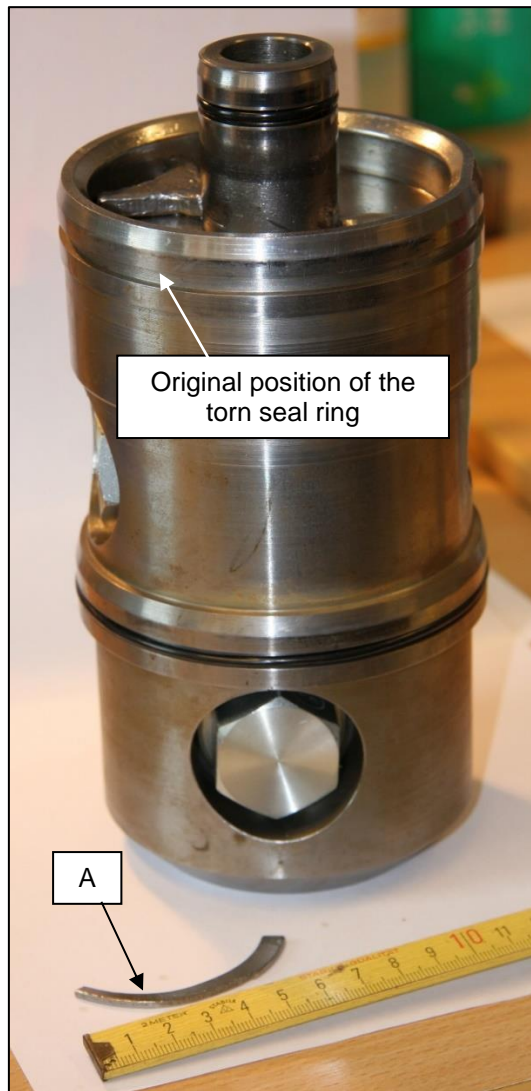
Figure 45: Valve body and removed foreign body (A) 27
