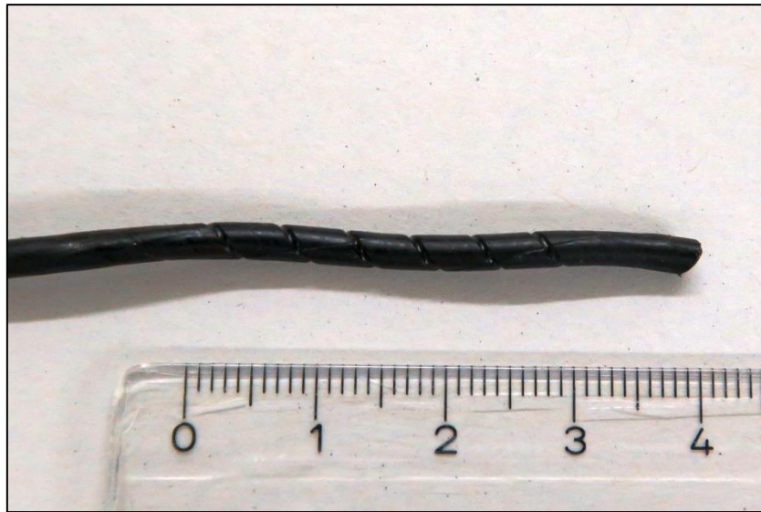
Figure 48: Torn seal ring with notches
