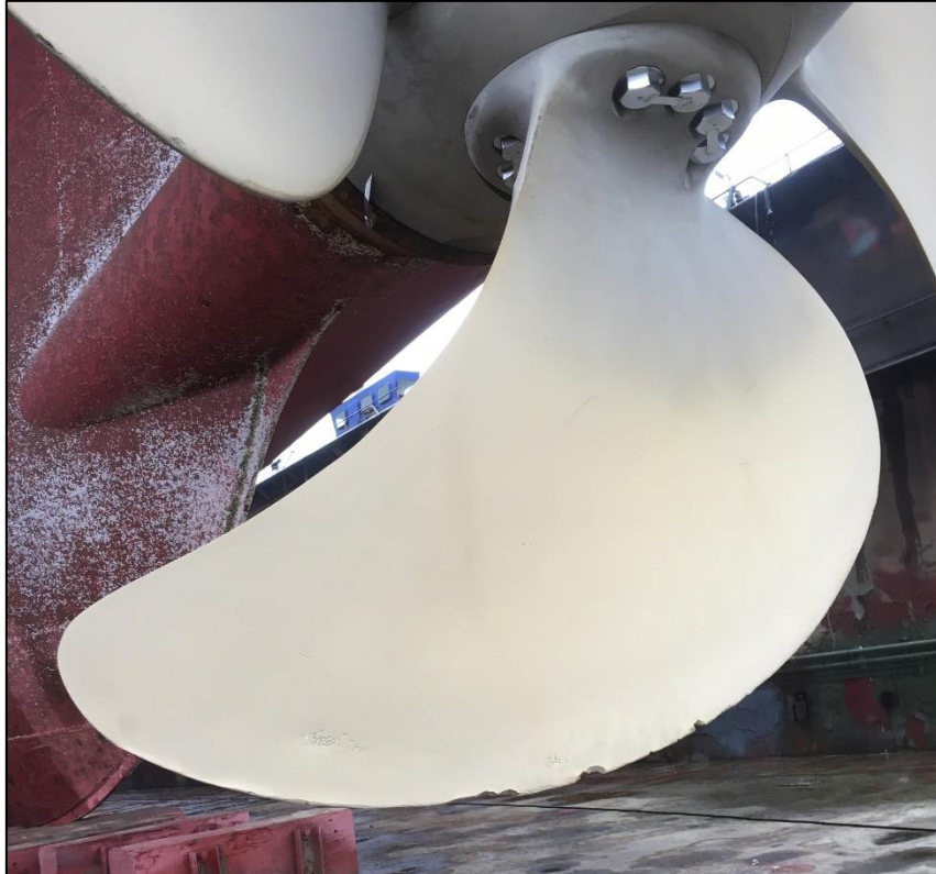
Figure 36: Damage to one of the propeller blades
