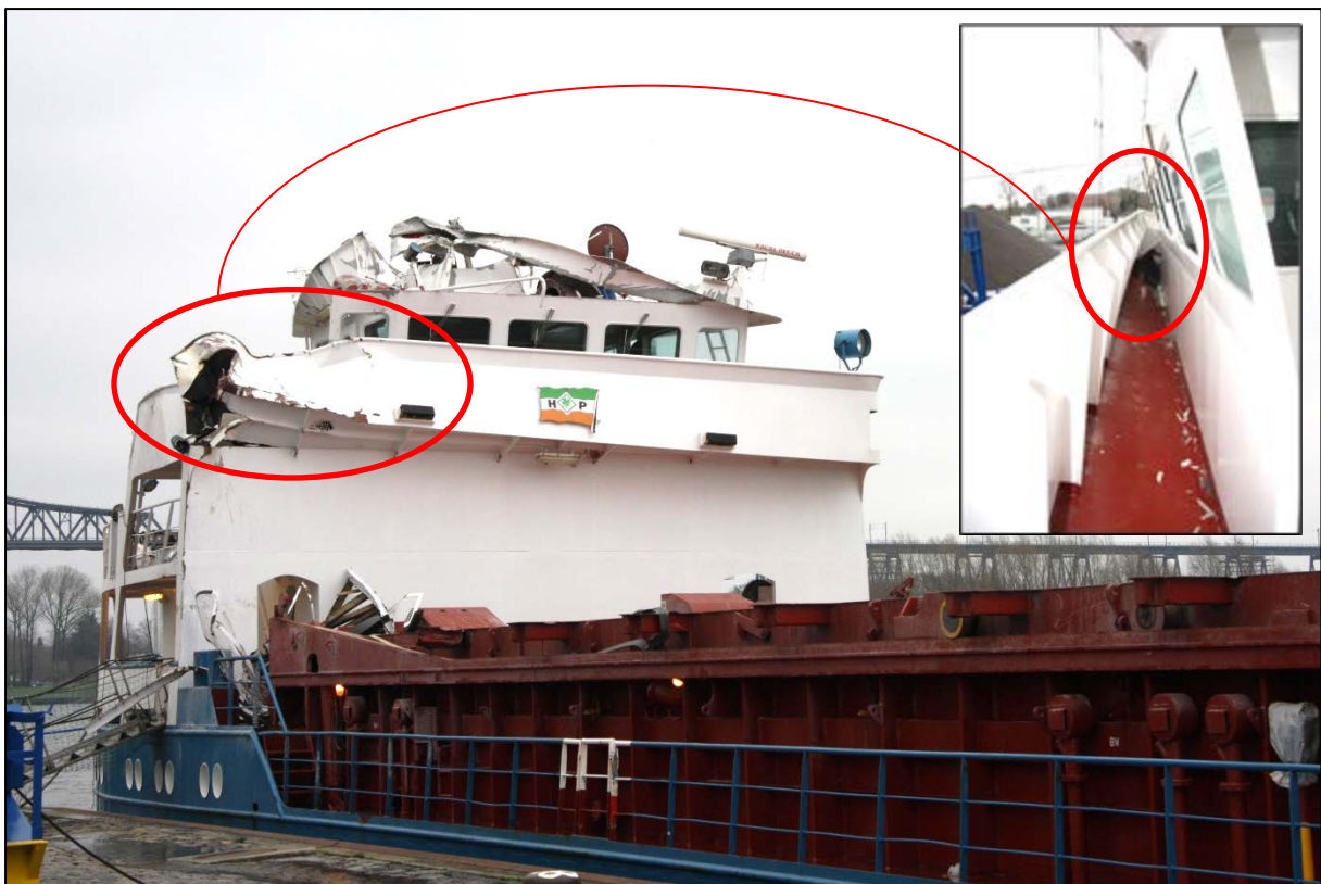
Figure 27: Overview – damage to the EVERT PRAHM's superstructure
