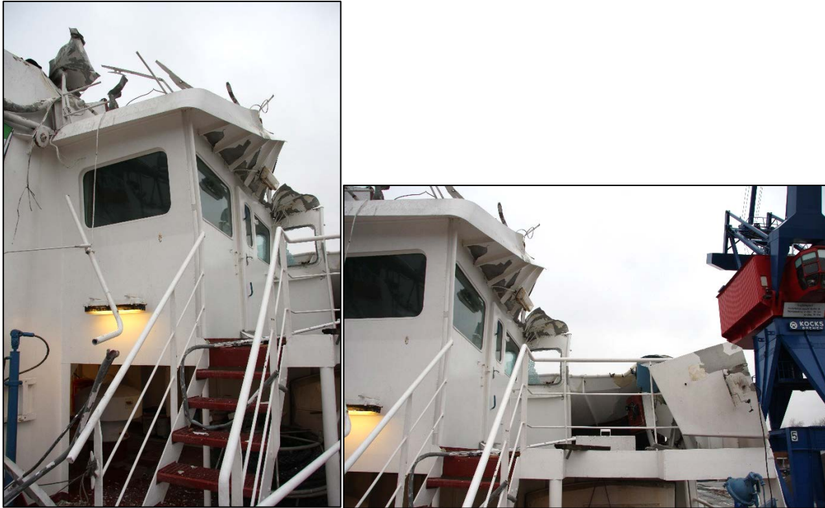
Figure 28: Damaged starboard wing on the EVERT PRAHM
