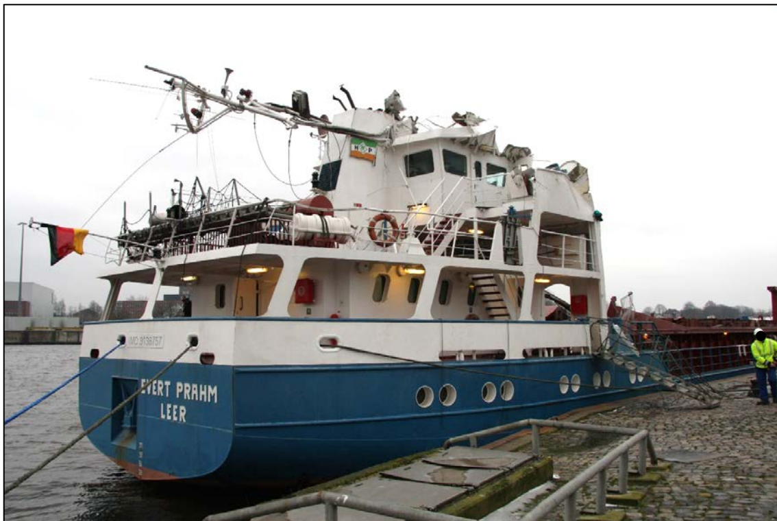
Figure 29: Damage to the EVERT PRAHM's superstructure, view from astern
