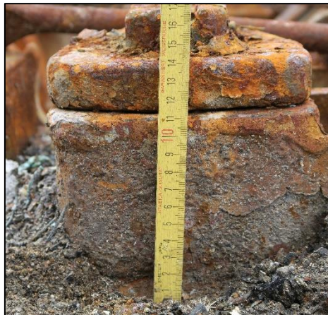
Figure 56: Height of container foot plus twist lock
