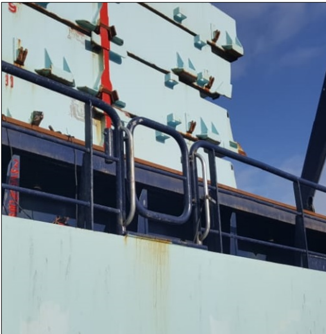
Figure 16: Handholds for accessing the deck of the MARFAAM (October 2019)
