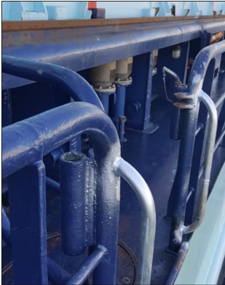
Figure 17: Handholds for accessing the deck of the MARFAAM (October 2019)
