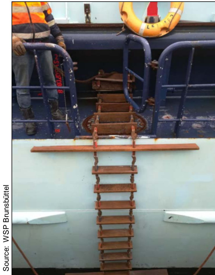
Figure 4: The MARFAAM's pilot embarkation point on the day of the accident
