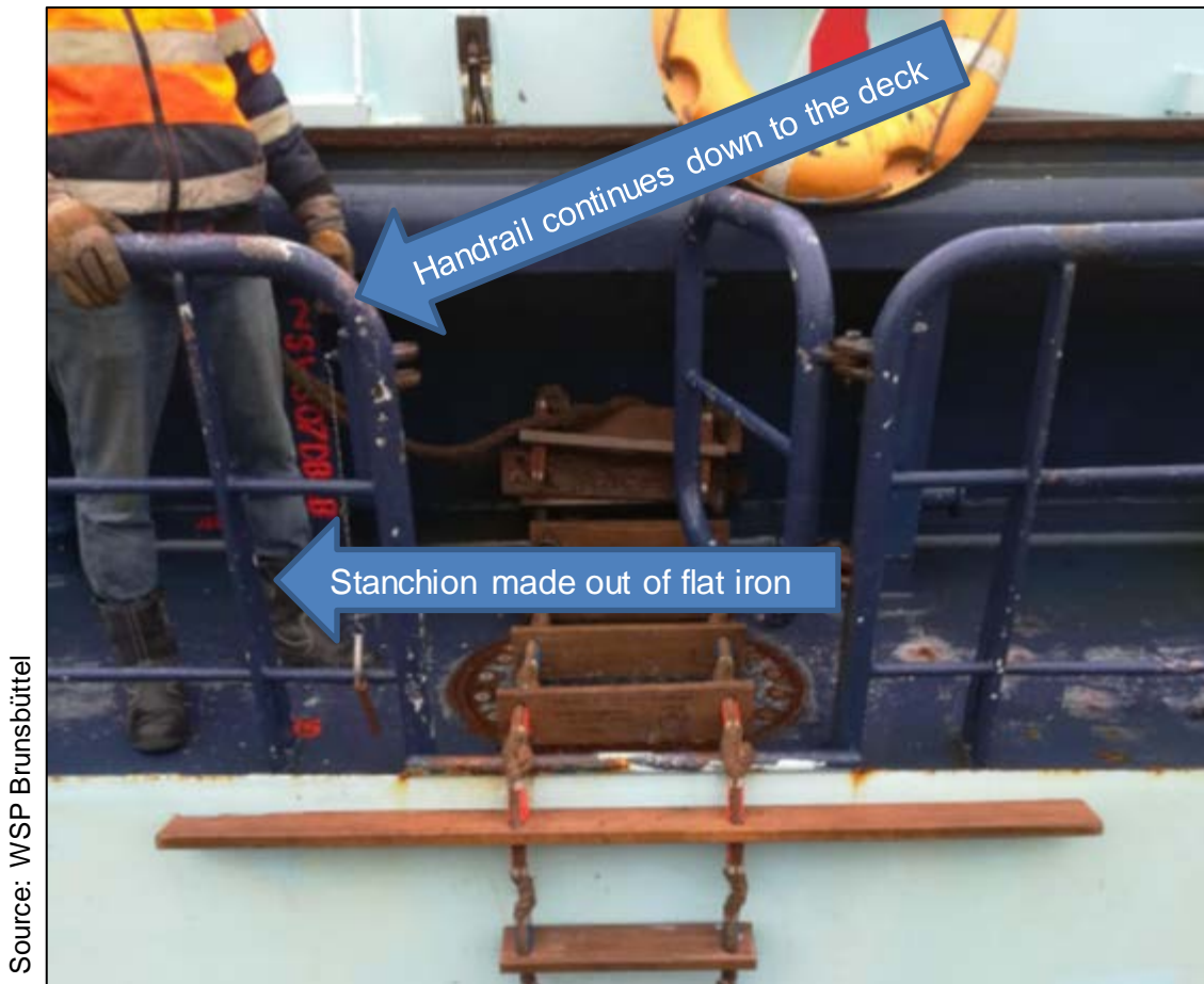
Figure 10: Handrail continues down to the deck
