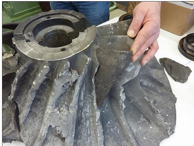
Figure 28: Deformed and broken compressor blades with material smearing
