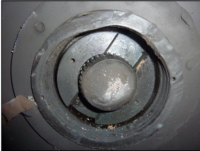
Figure 18: Fracture surface on the shaft with fatigue fracture
