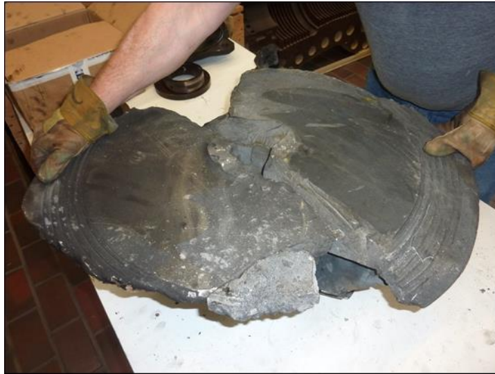
Figure 27: Rear of the compressor wheel with sealing labyrinths
