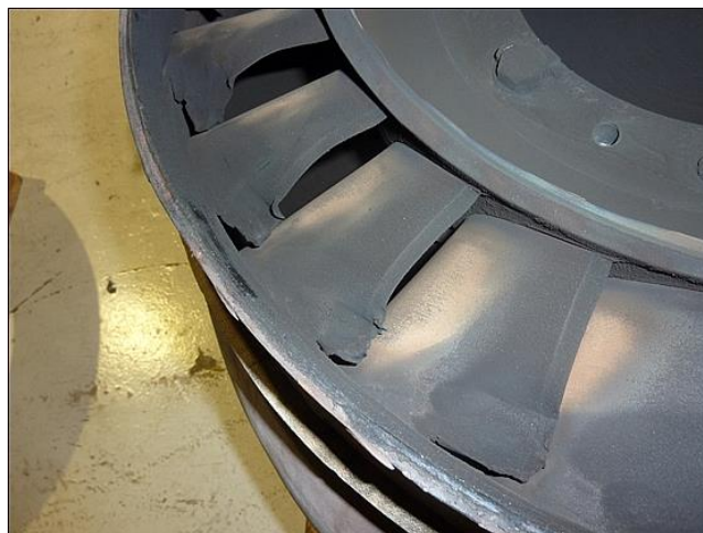
Figure 25: Damaged nozzle ring
