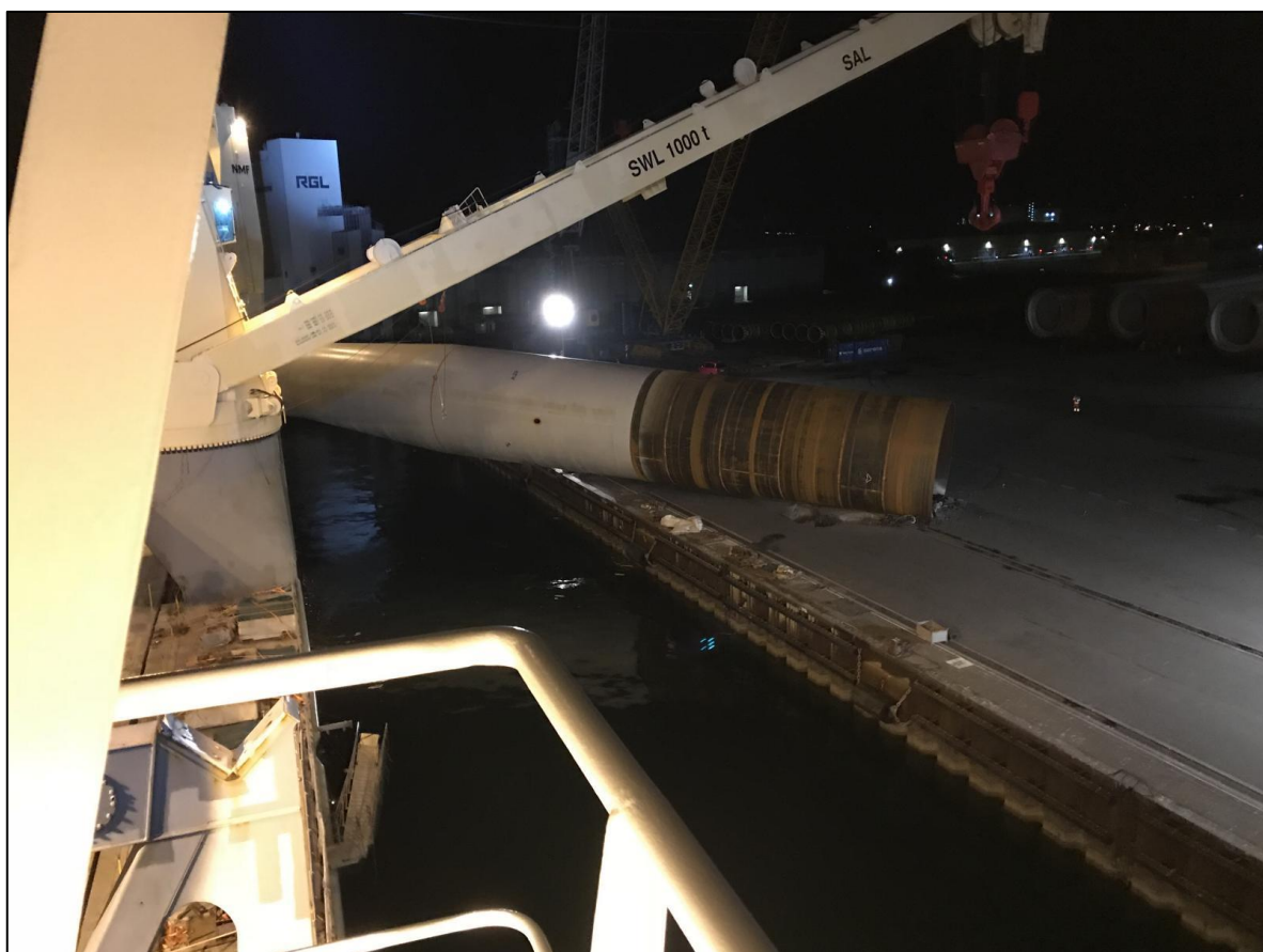
Figure 12: Final position after the MP slipped
