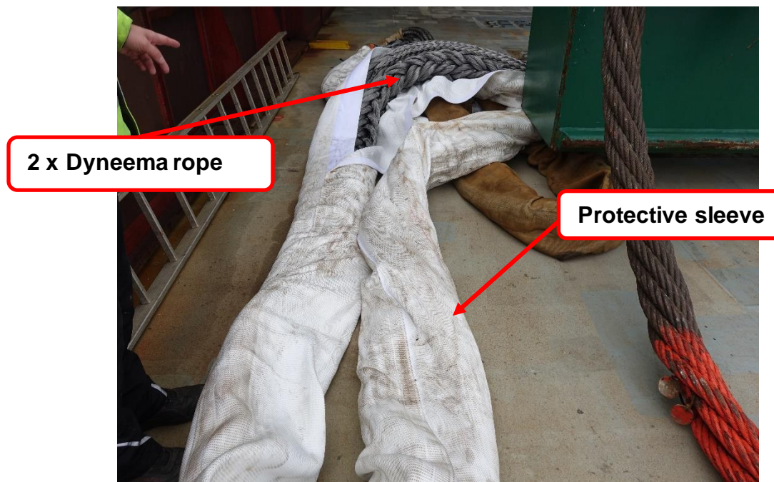
Figure 15: Lifting sling from the conical part of the MP
