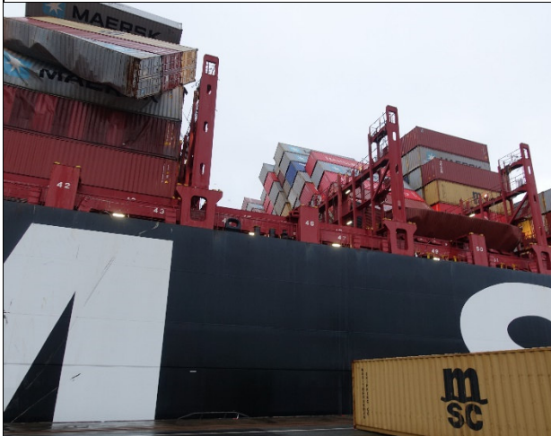
Figure 9: Collapsed rows in bay 42 and 50. (Source: BSU)
