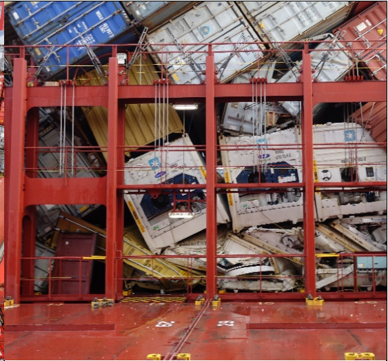
Figure 8: Collapsed containers in bay 26. (Source: BSU)
