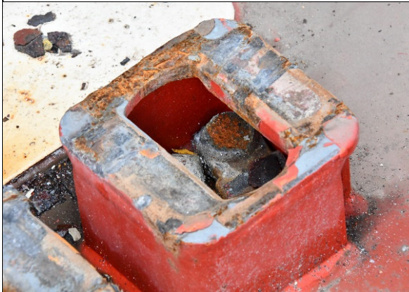
Figure 15: Broken twistlock in a bent deck fitting (Source: German Waterway Police)
