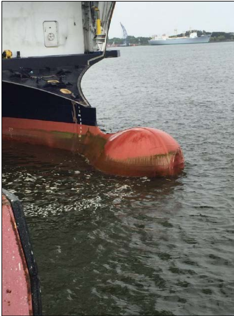
Figure 8: Deformation of the bulbous bow to port
