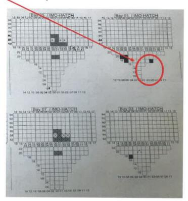
These areas are normally only "single stowage positions", which are neither used for breakbulk, nor can be entered accidently, due to their open construction. Therefore, we do not deem it necessary to install a "tiger" marking as mentioned above. However, all other measures are also applicable for the forward locations.
