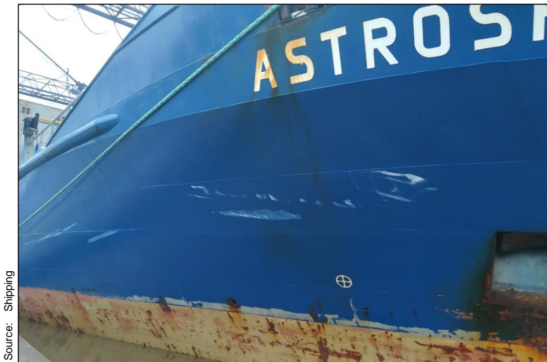
Figure 8: Close-up view of the damage to the ASTROSPRINTER
