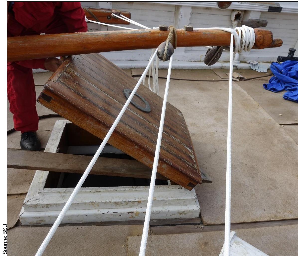
Figure 64: Aft hatch blocked by the tiller
