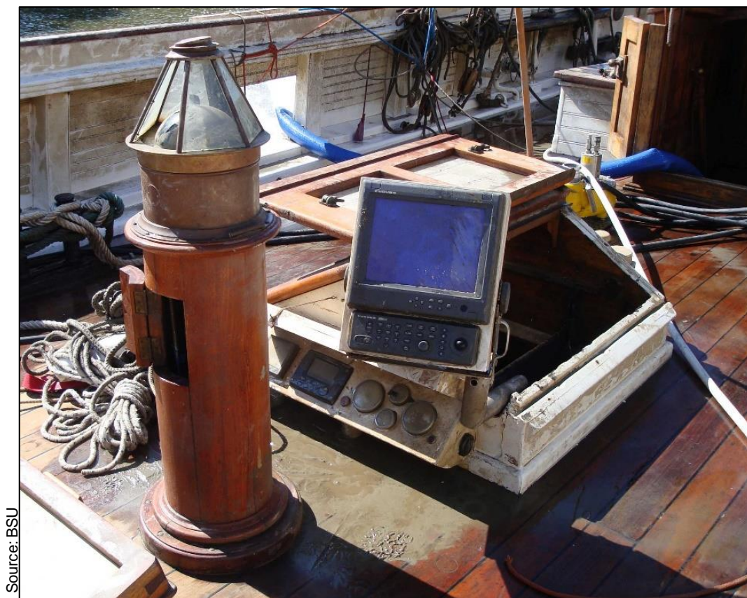
Figure 11: Combined radar and chart plotter at the steering position
