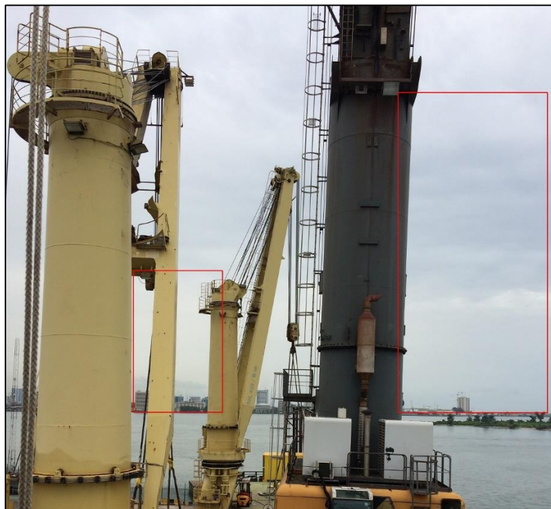
Figure 23: Loading of LHM 550 cranes on the following voyage (view of horizon) The insertion of rectangles shows that although the ship was not heeling (own cargo-handling gear, left, is at a right angle to the horizon), the loaded crane was still inclined (right; no right angle)
