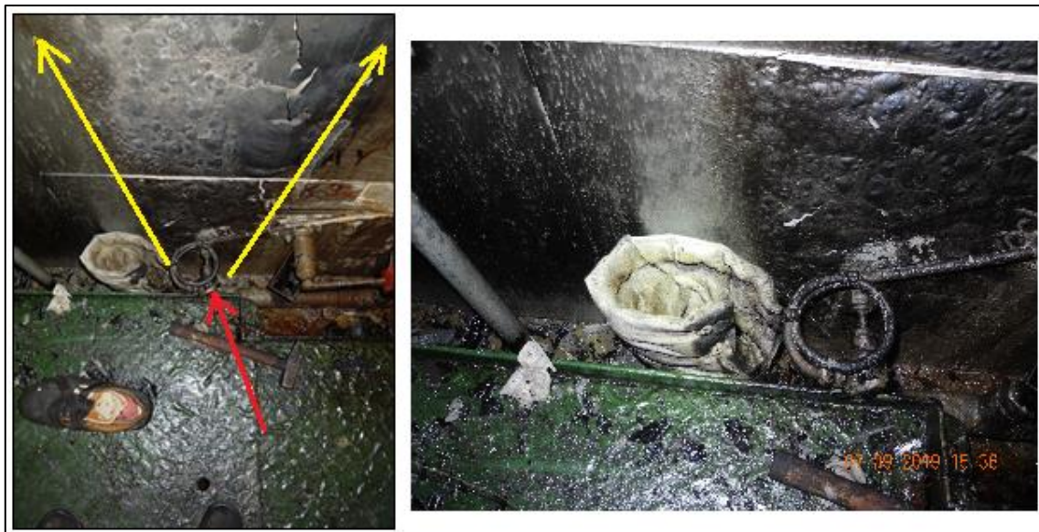
Figure 22: Position at which the fire funnel starts
