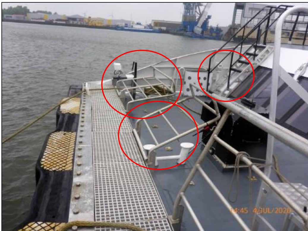
Figure 5: Damage to the SEEWIND I's fore section 9
