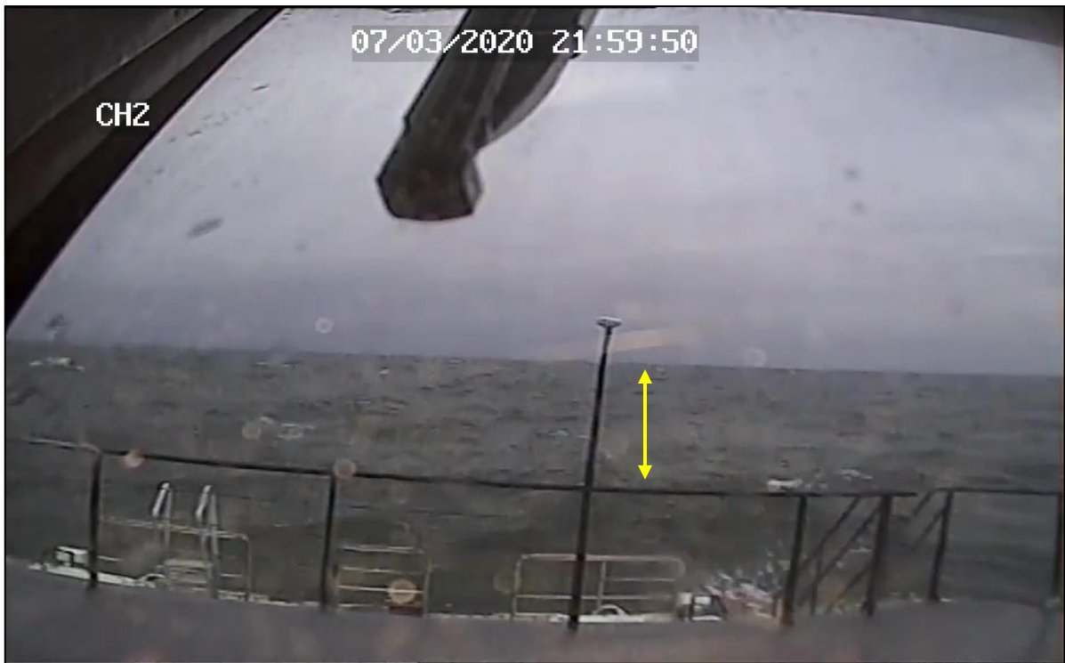
Figure 13: Front camera screenshot at 215950 The bow drops further than usual (see also Figure 12).
