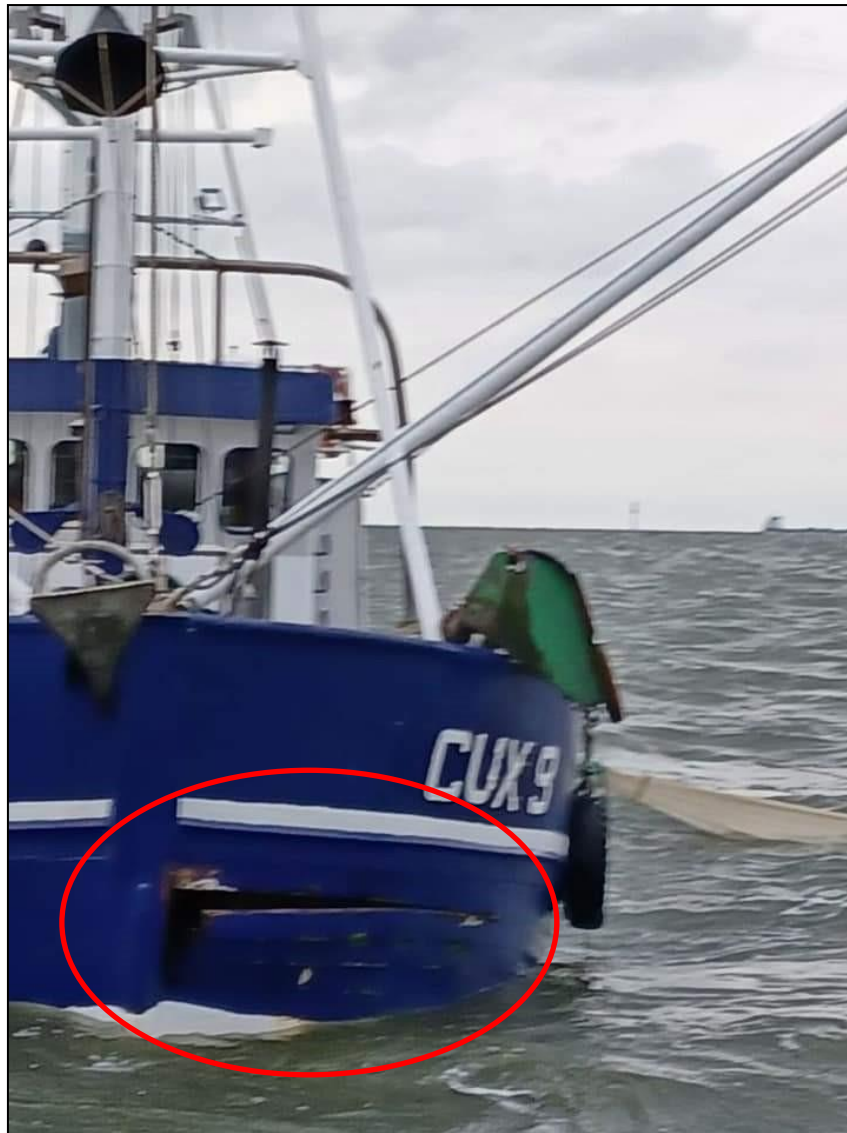
Figure 3: The loose planks at the bow of the RAMONA 5
