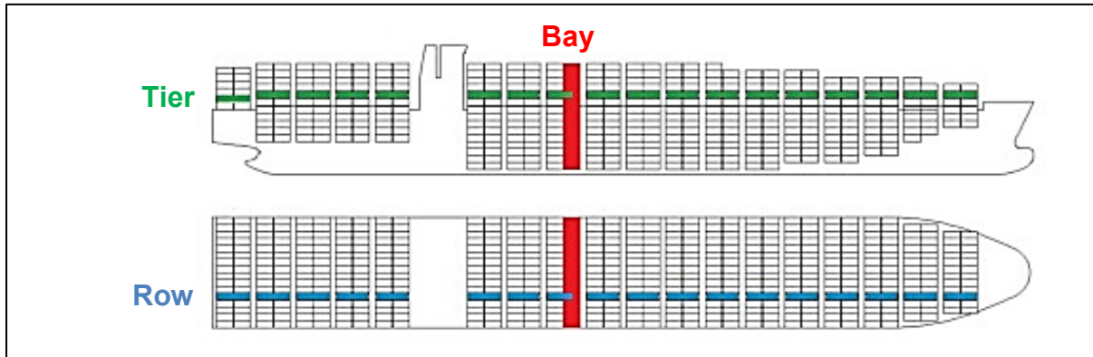
Figure 3: Diagram of Bay-Row-Tier System on Container Ships 12
