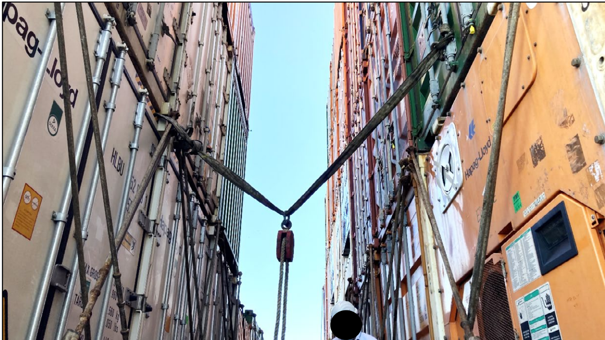
Figure 15: Rope and Snatch Block System for Evacuation via the Access Hatch (reproduced on 19 October 2021) 80
