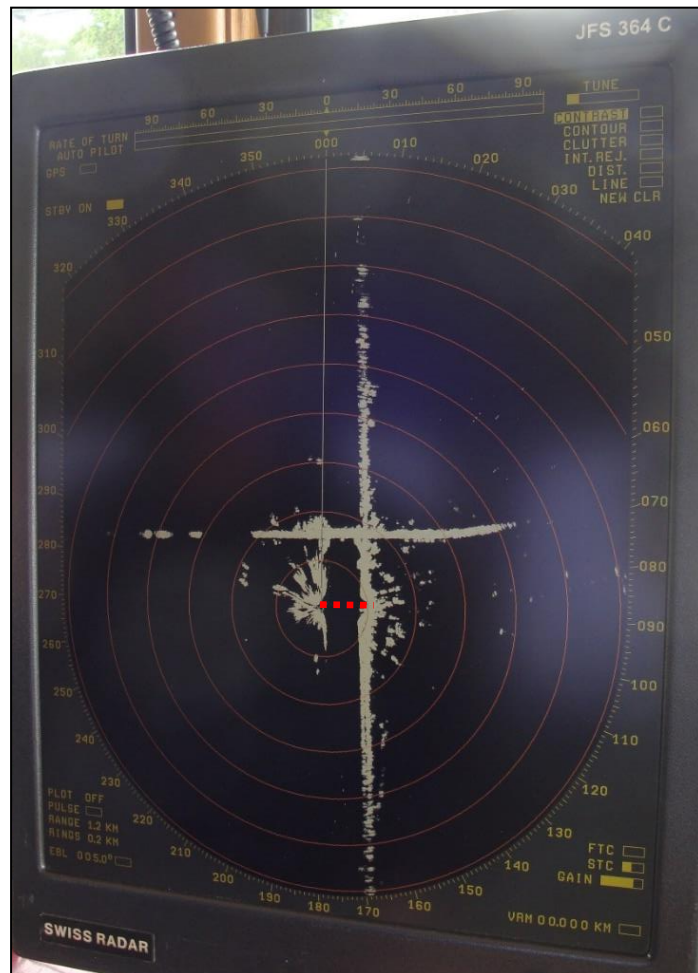
Figure 19: Radar image (the AUDORF), range = 1.2 km 36
