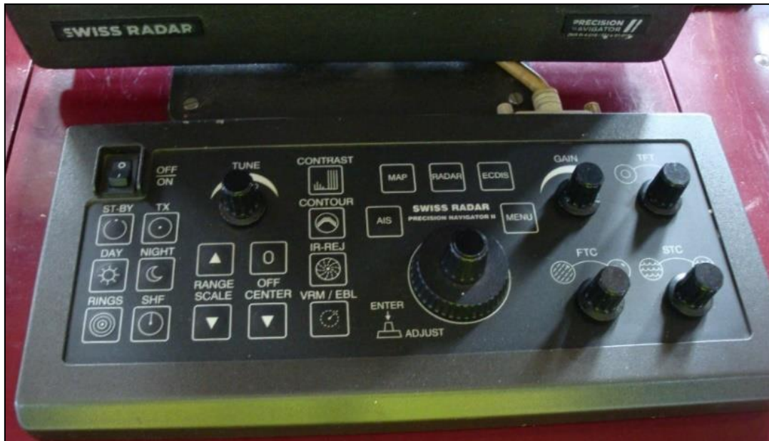
Figure 18: Control panel for the radar set on the HOCHDONN 35
