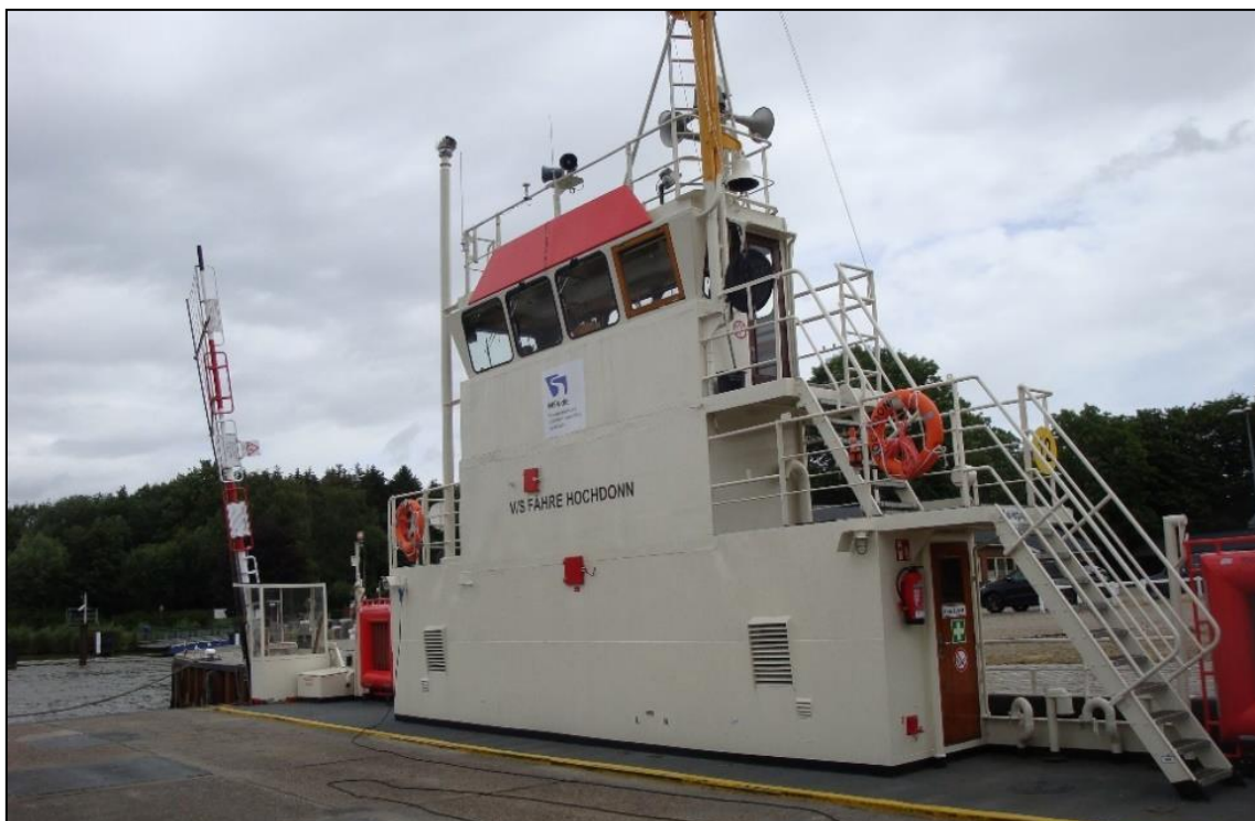
Figure 9: Side deck superstructure with bridge operator stand
