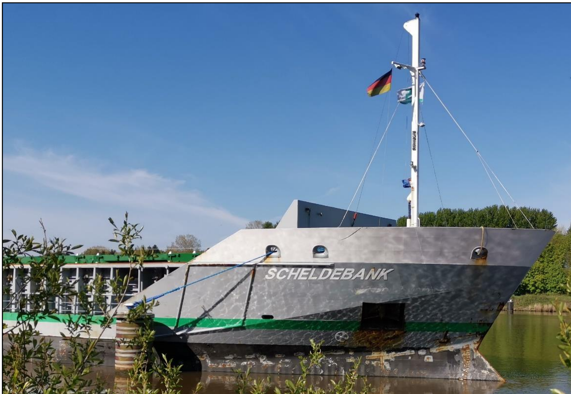
Figure 4: Paint abrasions on the starboard bow of the SCHELDEBANK 14
