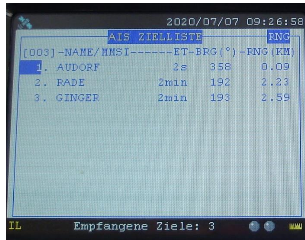
Figure 36: AIS target list on the HOCHDONN (0926)
