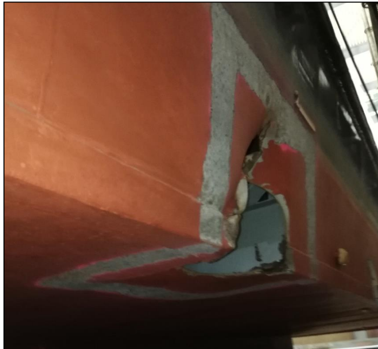
Figure 8: Hole in the HOCHDONN's hull 18
