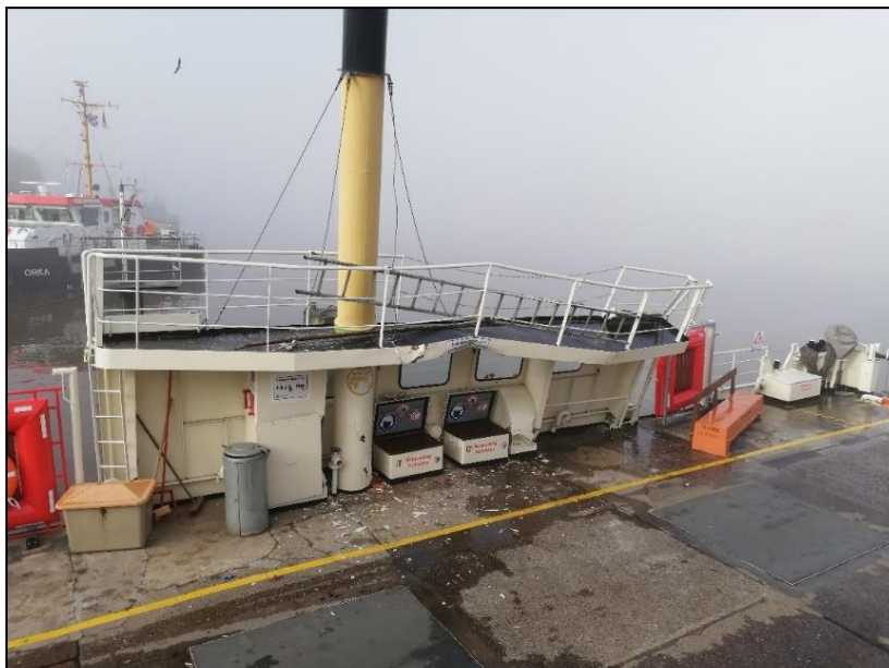
Figure 6: Damage to the ferry's starboard side 16
