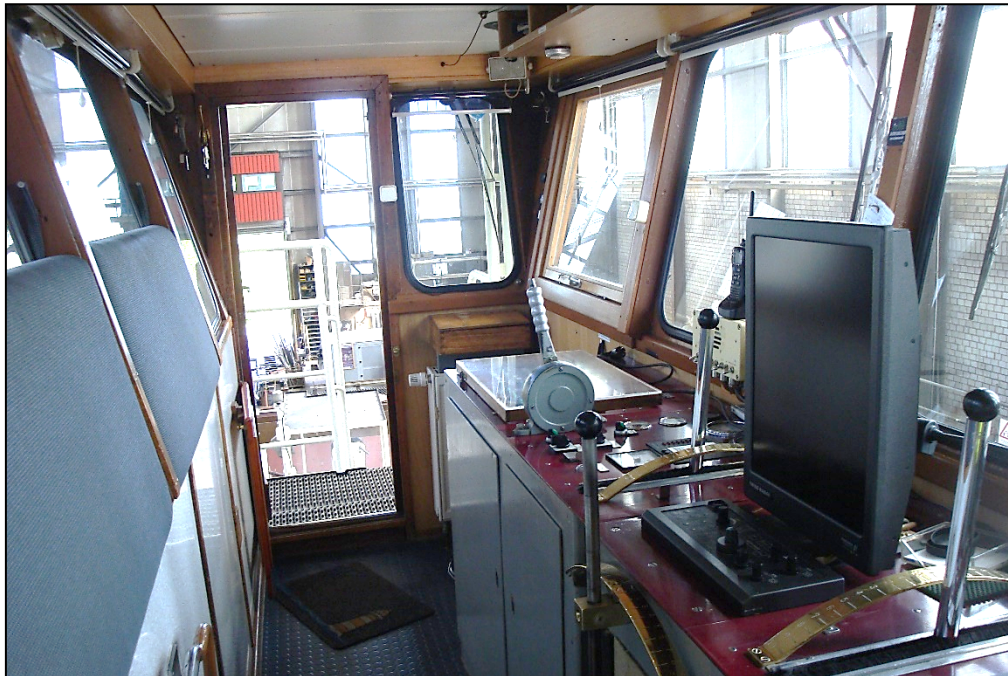
Figure 10: Control position on the HOCHDONN with lever control (view towards the bridge door)
