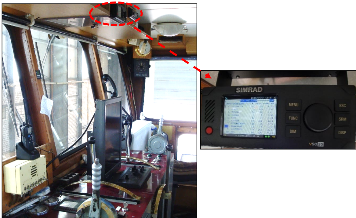
Figure 23: AIS device above the steering position
