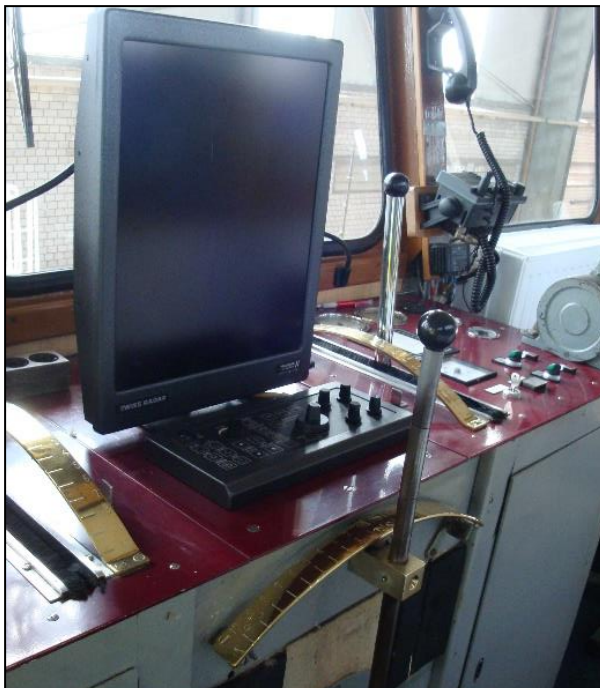
Figure 16: Radar set (control position on the HOCHDONN)
